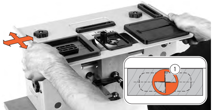
3-23 The jig table is centered over the marked workpiece with the sight ①.
