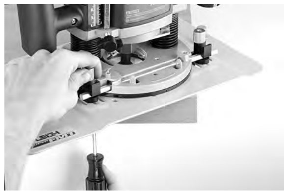
2-20 Slide the router/sub-base assembly on the corner of the bench so that one clamp screw is overhanging the edge. Loosen this screw just slightly. Push the sliding washer in to touch the router base, and holding it in position against the router base, tighten the screw firmly.
