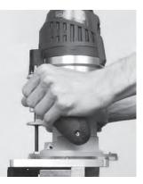
**3-5** Do not tilt the router on the jig. Keep the router flat on the jig assembly.
