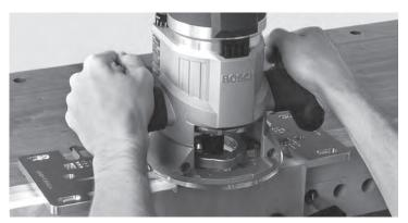
**3-6** If you insist on removing the router from the jig while it is still revolving, always pull it straight off the jig horizontally, and do not raise or lower the router until it is completely clear of the jig.
