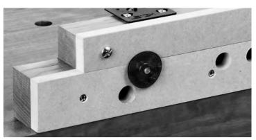
**1-22 Optional Hold-down for Bench Use** Notch out the ends of the beam in order to clamp beam assembly to a bench and use in hand-held router mode.
