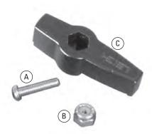
**1-9 Assemble the Latches** There are three parts to each latch assembly: the latch screw (a), the nyloc nut (b) and the plastic latch (c). Press the nyloc nut into the hexagon opening in the top of the plastic latch with the white nylon insert facing up. Next, screw in the latch screw from the bottom of the latch. Do not tighten the screw at this time.
