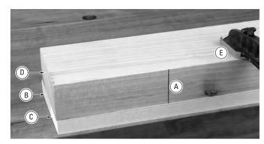
**1-5 This procedure is critical to the accuracy of the jig.** Before attaching the MDF boards to the beam, use each pin plate as a drill guide. First, mark a line  $4\frac{1}{2}$ "[114mm] in from the left end of the **top of the beam** and square it across (a). Next, stack the clamping surface (b), sacrificial board (c) and beam (d) near the edge of the workbench and clamp in place (c).
