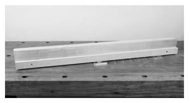
**1-13** Turn the assembly upside down. Take a piece of the predrilled sacrificial board and lay it flush on the template.
