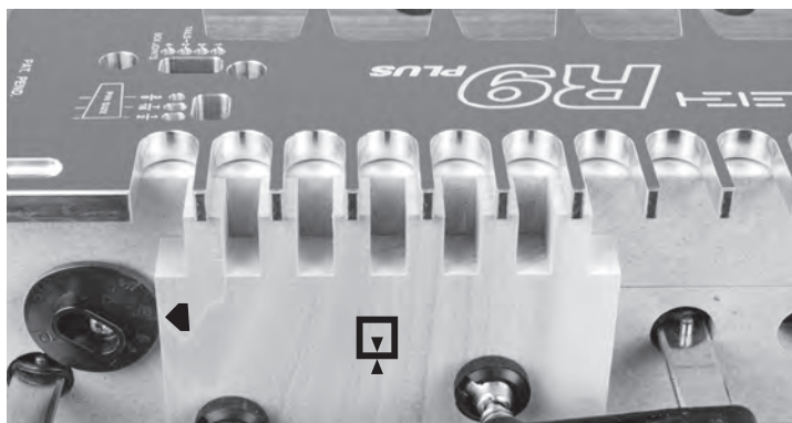
7-12 Rout all of the sockets. Remove socket board.
