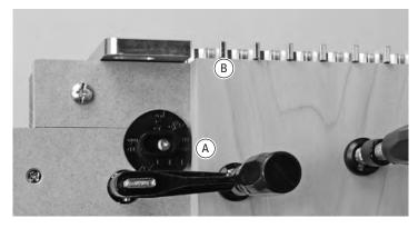
**4-4** Boards are always clamped against the sidestop (and flush under the template (B).
