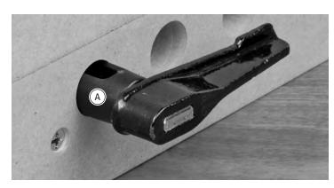
**4-3** Squeeze the tips of the clamp locator (a) and insert through a clamp hole in the beam. Clamp locators hold the clamp arm firmly in place while the clamp's screw arm is attached from the opposite side of the beam.
