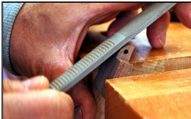
Fine-tuning curvature, to provide turning clearance.
