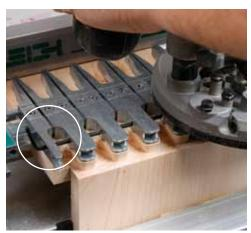
**Clever engineering.** For half-blinds in one pass, a rod slides through the template fingers to stop the bushing's rearward travel in the right spot.
