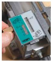
**Short learning curve.** Icons tell you which way the template goes on the jig, and precise guide lines dial in its position for any stock thickness.
