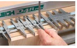
**Magic fingers.** All you need is a center mark to design the array of pins (left). You can trust your eyes from there, and even if the symmetry is off, the design of the template ensures a perfect match between pins and tails when you flip it (below).
