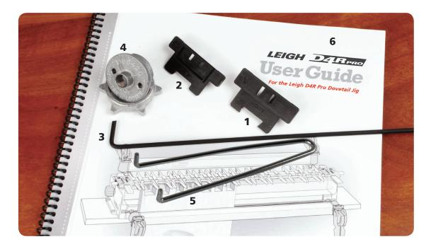
\*In addition to the parts shown above, you will need to modify the tail end of each guide finger as described on the following pages. *Note: No modification is required for finger (box) joints.* **If you would prefer a "new" set of D4R Pro fingers, see "D4R Pro Guide Finger Set" at www.leighjigs.com/jig-upgrades/ for details.**
