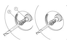
Check the shank size of each cutter selected, then use the appropriate collet ① or collet reducer ②. 1/4" collet reducers come standard with most 1/2" collet routers, but
