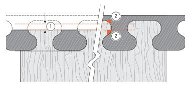
**9-2** The ideal thickness range for through Isoloc boards is 7/6"[11mm] to 9/6"[14mm] ①; perfect for drawer sides to drawer rears, or for small to medium boxes. Anything more or less than these thicknesses could cause tear-out problems at ②.
