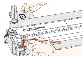
**9-4** Mount a scrap piece of exactly the same thickness as the pin board in the front clamp, slightly below the top surface. Remove the spacer board. Clamp the through socket board horizontally in the rear clamp, inside face  $\Box$  of the board away from the jig body and the end edge flush with the outer edge of the vertical scrap board. Lower the template flush and level onto the socket board.
