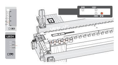
**9-5** Set the template on the socket **TS** icon. **Set the scale on** 17mm (there is no precise equivalent setting on the inch scale). Now rout a test socket board.
