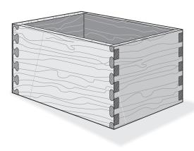
**9-1** Although intended primarily as a half-blind joint, the Isoloc can easily be used for attractive through joinery. This is particularly suitable on the rear corners of drawers where the same Isoloc pattern had been used on the drawer front.
