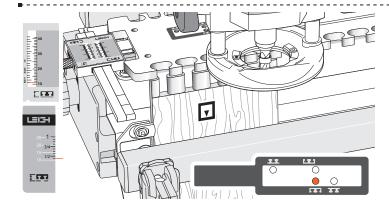
**9-3** Routing the through pins is straight forward. Set the template on the pin  $\square$  icon and the scale on **the actual pin board thickness** (shown here at  $\frac{7}{16}$ "[11mm]). The inside face  $\square$  of the board is away from the jig body as before.
