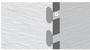
**9-6** The ends of the socket board should slightly project through the pins ① for cleanup after gluing. Move the template in for more socket board projection; out for less projection. The 17mm scale setting works for all through pin board thicknesses.
