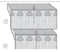
**10-1** Isoloc joints are template-made joints, but they are only symmetrical if the pattern appears to be even about the board centreline.
