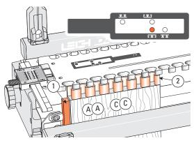
**10-6** Rout pins for corners A and C blocked away from the left side stop 1 so that the right edge finish 2 mirrors the B and D left edge finish in 10-5.
