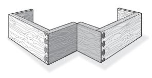
**10-2** Symmetry is not critical when only one corner can be seen at one time; as in this "split" drawing of a typical drawer front and sides.
