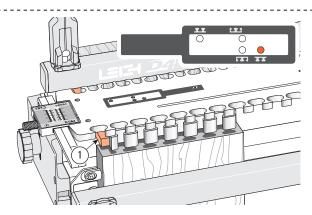
**10-7** Use the same block 1 to space the A and C socket boards away from the rear stop.
