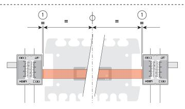
**1-6** The template bar must now be centred between the two scale assemblies ①. The following instructions show how to do this.
