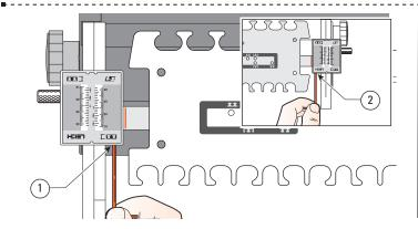
**1-9** Taking care not to move the template and template bar, tighten first one scale bar screw ①, then the scale screw at the other end ②. The template bar is now centred.
