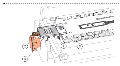
**1-5** Slide the template assembly onto the jig support brackets with the set screws ① toward you and lower the completed assembly gently onto the spacer board ③. Tighten the support bracket knobs ④. **Do not tighten the set screws** ①. Make sure the scale reading is the same on both scales, say on the 1"[25mm] mark, then tighten the thumb screws ②.
