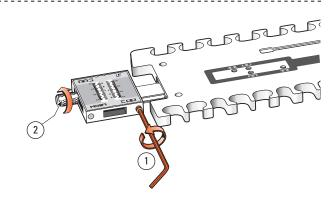
**1-4** Loosen the two scale bar set screws ①, and the two scale thumb screws ② at both ends of the template.
