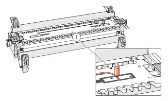
**1-7** Discard the plastic shipping plug from its hole in the template. Move the template until you can insert the template pin through the rear right hand hole ① and into the bar.
