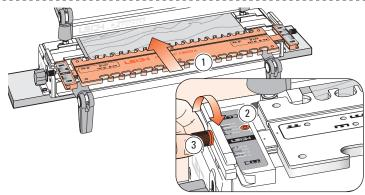
**1-12** Slide the finger assembly onto the support brackets, in the "single" joint pattern (key, clover or ellipse) to the front ① and the scale lock screw to the rear ② and set on  $\frac{3}{4}$ "[20mm]. Tighten both thumbscrews ③.
