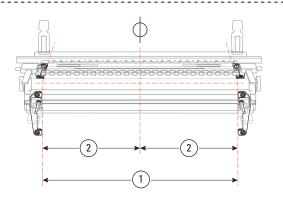
**1-3** To ensure the accurate joints your Leigh Isoloc was designed to produce, check that the jig side stops are correctly positioned as per the original jig body instructions, i.e.  $24\frac{1}{8}$ "[613mm] apart ① and equidistant from the centreline ②. D4R side stops are machined as part of the body.
