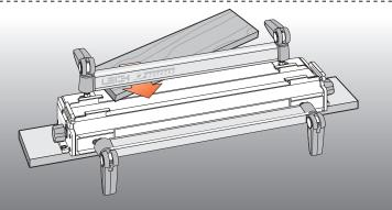
**1-10** Mount a Superjig or D1600 jig body firmly to a bench as per that jig's instructions. Clamp the spacer board into the rear clamp.
