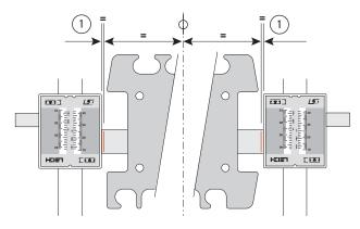
**1-8** Move the template with its template bar left and right in the scales until **the scored lines at each end of the bar** are approximately equidistant from the scales ①. You can do this by eye; the human eye is an excellent comparator. If the gap appears the same, it is close enough. If you're more comfortable using a rule or dial caliper, by all means use it. *Note: The scored lines are illustrated in red for clarity.*
