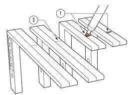
**1-2** Support Bracket Markings D1258, D1258R and D3 jigs have short brackets marked with an 'arrow' for scale line-up. Shade the arrows with a black felt pen ① for better visibility.
