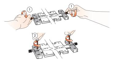
**1-11** Mounting I1600, I18, and I24 Isoloc Templates Install the two thumbscrews a few turns into the scales ①. Loosen the scale lock screw ② at both ends (by one turn only).
