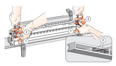
**1-14** Taking care to not move the template, pull up on the template bar ① while pushing down on the scale ② to ensure the bar is touching the two registration pads ③ inside the scale. Maintain pressure and tighten the scale lock-screw. Repeat at the other end. The template is now centred.
