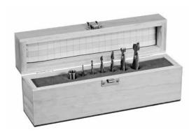
1806F High Speed Steel Boxed Bit Set, 7 pc Features 5 two-flute HSS spiral upcut bits and 1 single-flute (Bit 163). Set includes bits 163 (3/32"), 164 (1/8"), 166 (3/16"), 168 (1/4"), 173 (3/8"), 180 (1/2"), and collet reducer 172-375.
