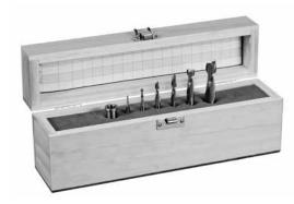
1806C Solid Carbide Boxed Bit Set, 7 pc Features 5 two-flute solid carbide spiral upcut bits and 1 single-flute HSS (Bit 163). Set includes bits 163 (3/32"), 164C (1/8"), 166C (3/16"), 168C (1/4"), 173C (3/8"), 180C (1/2"), and collet reducer 172-375.
