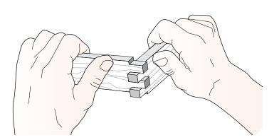
**9-3** Test for fit. Don't worry about board alignment, it's only the fit you're testing. Adjust the **e-Bush** by trial and error and rout more pairs of scrap board ends as required.
