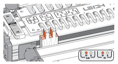
**9-2 Quick Fit Test** Rather than routing test pieces separately, here is a quick way to get 99% of the way there. Simply rout two thinner boards of scrap stock simultaneously. Any single pin position will do, unless you intend to rout small box joints, in which case, use the matching pin positions described in chapter 8. If you prefer, use one piece and saw in half after routing.
