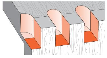
**9-1** To help prevent tear-out on the sides and bottom of the exit cut, back up the cut with a horizontal board end-grain pushed against the back of the workpiece and held in the rear clamp.
