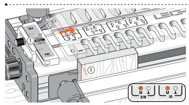
**7-3** Set the template pin on **U**. Clamp a scrap piece vertically in the jig front with its top end slightly above the jig body ①. Clamp a box front horizontally with the inside face **□** away from the jig body, and the front end edge against the scrap board.
