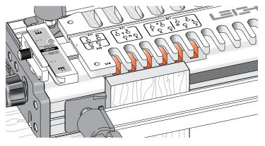
Rout a test piece to test the scale setting for joint flushness and adjust the template in or out to produce the required flush
