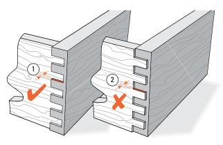
**7-6** The drawer front pins should project through the side sockets by no more than 1/64"[0,25mm] for clean-up ①. If the sides project 2, adjust the template inward to suit.
