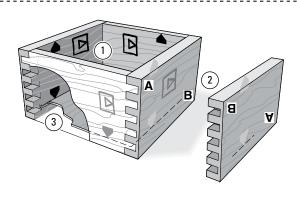
**7-8** Square half-blind box joint boards must be assembled with the inside faces inwards ① but unlike normal box joints, the sides edges may be up or down ②. So you can decide on the preferred board orientation before marking and routing the box bottom grooves 3. You will probably need to clamp in both directions when gluing-up.
