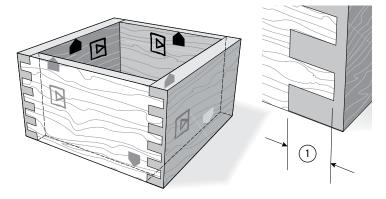
**7-1 Half-Blind Joints** Unlike normal box joints, the inside faces of half-blind box joint boards always face away from the jig body, and alternate edges are placed against the side stop. Set the depth of cut ① to about ½"[3mm] less than the drawerfront thickness. Use only the "Symmetrical" board widths for half-blind joints.
