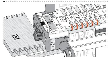
When satisfied with the flushness fit, rout all the ends of the box fronts and backs in this mode.
