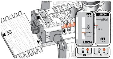
**7-2** Set the template pin on the **1** setting and the scales to the thickness of the box sides, e.g. <sup>3</sup>/<sub>4</sub>"[20mm] shown here. Rout the box side ends vertically in the front clamp.
