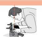
Reading scales from directly overhead improves setting accuracy.
