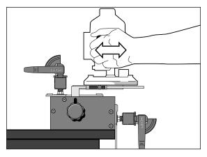
**2-9** Keep the router flat on the jig assembly.
