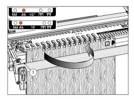
**6**. Turn board No. 1, like turning the page of a book so the side stop mark is now to the right. Very carefully position and clamp the board in the jig so the previously routed sockets in the workpiece perfectly line up with the routed sockets in the backup board. Keep the left edge of the board away from the side stop ①. Rout the left side of this end.
