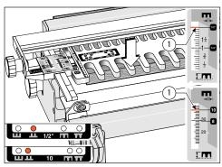
**2**. Lower the template onto the backup board and set scales on the comb size to be used (example here: ½"[and 10mm] combs ①). Position the template with the template pin in the **4** position.
