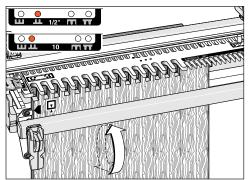
**5**. Rout the full width of the active comb on both ends of boards 1 and 3 in position **1**. Be sure to keep the same side edges to the side stop. **Do not move or remove the backup board.**
