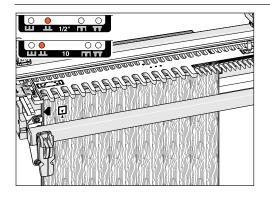
**4**. Clamp board No. 1 in the jig, side edge mark to side stop, top end edge touching the underside of the template. Make sure the horizontal scrap board is touching firmly against the rear of the workpiece.
