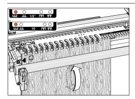
**8.** Rout both ends of boards 2 and 4, first routing both ends of each board against the the left side stop, and then...
