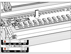
7. Move the template to position **u** and replace the backup board with a new clean-edged piece.
