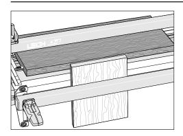
1. Replace the spacer board with a scrap backup board. This board needs to be flat and even thickness like the spacer board and have its front edge straight. It should be long enough to extend past the end of the active comb. Clamp a temporary front board and position the backup board touching it. Clamp the backup board and then remove the front board.
