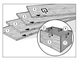
**3**. Refer to the extended board width chart on the back of this bulletin. Prepare four boards and mark them 1,2,3,4. Select the grain alignment and mark the common top (or bottom) edges. Don't worry about face side selection, this can be done after routing.
