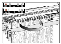
**9**. ...reposition (as with boards 1 and 3) to align and complete the routing. **Keep the left edge of the board away from the side stop** ①. Rout the left side of this end of boards 2 and 4.
