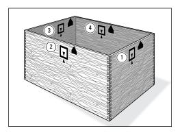
10. Keeping the marked side stop edges of all boards toward the top (or bottom) of the box, select the preferred outside faces of the boards and assemble the box. Remember; box joint corners need clamping from both directions, or use strap clamps and blocks.
