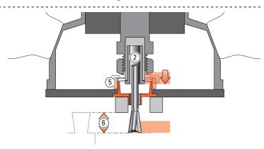
**7-4** Tighten the collet ② securely and lower the collet to adjust the depth of cut ⑥, but make sure the collet does not contact the guidebush ⑤.
