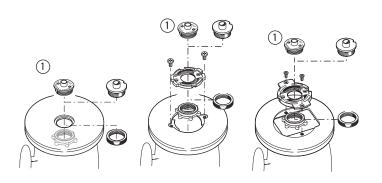
**7-1** Fit the e7-Bush ①. One is included with your Super Jig. Some guidebush adaptors may have to be modified to allow adjustment rotation of the e7-Bush in the base. *See page 67*. If the e-Bush is incompatible with your router, any 7/16"[11,1mm] guidebush (min. depth ½" see page 67) will work for all but box joints on the Superjig.
