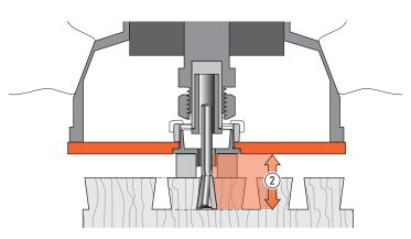
**7-6** Depth of cut is **not** the distance the bit projects from the router base. This is bit projection 2. This user guide generally refers to depth of cut. Bit projection ② is always .500"[12,7mm] more than depth of cut.
