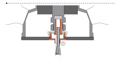
Ideally, the router collet (and bit) should be concentric (centered) to the guidebush as in figure 7-5. Regrettably, this is often not the case; the bit can be off center (eccentric to) the guidebush ①. The illustration shows the problem highly exaggerated. The good news: bit to bush alignment doesn't affect joint fit or flushness; both are "adjusted out" in normal jig setup.
