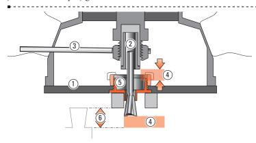
**7-3** When fitting a bit to the router ①, fit the shank as far into the collet ② as possible. Always rout with the collet as close to the guidebush as possible. Usually you can't securely grip the collet nut with a wrench ③ if the collet is at its optimum low position. Fit the bit so that the remaining travel ④ between collet and guidebush ⑤ will let the bit reach the required depth of cut ⑥.
