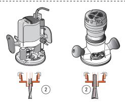
**7-8** Bit to guidebush offset may change when the router motor is unclamped from the base when changing bits or making bit height adjustments. Concentricity problems can also arise if two routers are used for through dovetails, (one for pins; one for tails). Routers with different bit to guidebush offsets 2 (misalignment shown highly exaggerated)...
