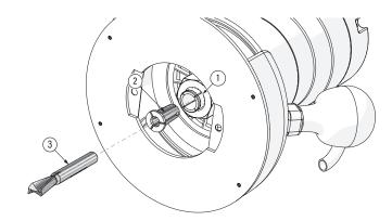
**7-2** Routers used on Super Jigs must have a ½" or 8mm collet ①. All Super Jig bits have 8mm shanks. Routers with ½" collets must use the ½" to 8mm collet reducer ② supplied with the jig. The collet reducer ② is inserted in the router collet ① (chuck) and the 8mm shank bit ③ is inserted in the collet reducer. Routers with 8mm collets do not require a collet reducer.
