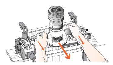
**5-6** If you insist on removing the router from the jig while it is still revolving, always pull it straight off the jig horizontally, and do not raise or lower the router until it is completely clear of the jig.
