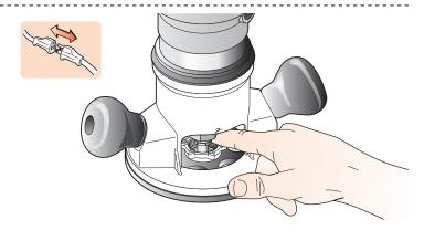
**5-4** Always disconnect the power source from the router when fitting bits or guidebushes, or making adjustments.
