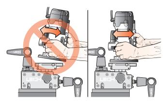
**5-5** Do not tilt the router on the jig. Keep the router flat on the jig assembly. Note: The optional Leigh VRS attachment prevents router tilting.
