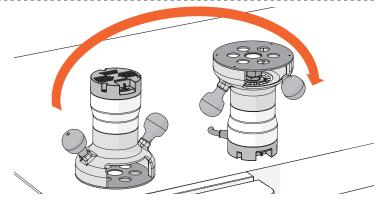
**3-4** To install the e7-Bush, follow these simple steps. Hold the router the way you normally hold and operate it on the jig. Now, up end the router in the same orientation.
