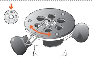
Use the pin wrench to align the No. 10 on the eBush to the reference line on the router base. The No.10 setting is used for all through and variably spaced half-blind dovetails on Superjigs. Settings for single pass half-blinds, box joints and sliding dovetails are described in applicable chapters. Be sure to retighten the e-Bush nut after each adjustment.
