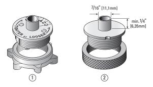
**3-1** The Leigh e7-Bush ① is used to rout through, half-blind, single pass half-blind and sliding dovetails on a Superjig. The elliptical design provides precise joint fit adjustment for box joints and sliding dovetails. A round 7/16"[11,1mm] guidebush ② (min. barrel length 1/4"[6,35mm]), can be used to rout through, half-blind, and sliding dovetails on the Superjig, but the e7-Bush is superior.
