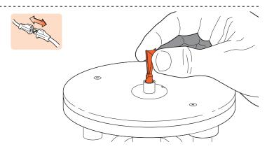
**3-8** The bit goes through the guidebush and fits in the router collet or chuck.
