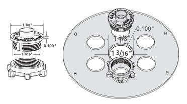
**3-5** To fit the Leigh eBush directly to your router, the router base must have a 1-3/8" diameter counter bore. If your router base does not have the correct counter bore, you will need a guide bush adaptor or aftermarket router base plate. Leigh offers several guide bush adaptors to fit many common routers. See the Guide Bush Adaptor Selection Chart in Appendix 1, page 68.
