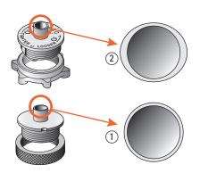
**3-2** The Leigh e7-Bush that comes with your Superjig is a unique template guidebush that is adjustable in size. Unlike regular circular template guidebushes ①, the e7-Bush is slightly elliptical in cross section ②. This simple innovation effectively changes the guidebush "active diameter size" when it's rotated, and provides benefits not possible with a standard round guidebush.
