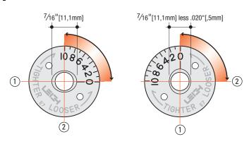
**3-3** The e7-Bush (7/16") fits the router base or a guide bush adaptor in the base (see Appendix I). The ellipse/oval shape has a major axis ①7/16"[11,1mm], and minor axis ②7/16"[11,1mm] less .020"[,5mm]. Turning the e-Bush 90 degrees in the router base changes the active diameter by .020"[,5mm] providing minute adjustment and recordable settings for perfectly fitting box joints.
