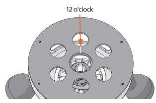
**3-6** Think of the router base as a clock face. Make a small scratch line or permanent ink mark on the router base or e-Bush adaptor at the 12 o'clock position ①. This will be your reference mark for all e7-Bush settings.
