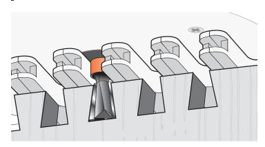
**3-9** The projecting part of the guidebush runs along the side edge of the guide finger. The rotating bit cuts the wood only, and touches neither the guidebush nor the guide surface.
