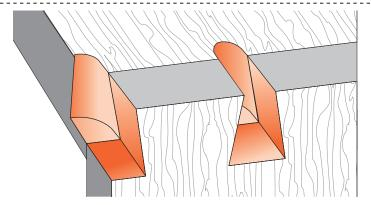
**15-8** To help prevent this, back up the cut with the end-grain of a horizontal board pushed against the back of the workpiece and held in the rear clamp. This board replaces the spacer board.
