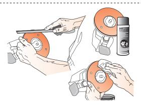
**15-16** Some router bases have sharp edges on the outside and inside corners. A slight chamfer of the edges with a fine file or sandpaper block will ease router movement on the jig.
