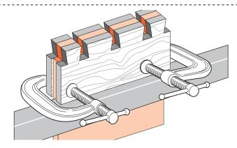
**15-10** For vulnerable or that last piece of exotic wood, clamp horizontal scrap pieces to the front and back of the work piece. Make sure clamps are below the bit depth.
