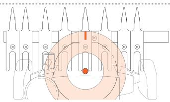
**15-15 Using The Router** Mark the router base top edge at the 12 o'clock position with a felt marker pen. Without wood or bits, try some dry runs in each jig mode. This will soon get you used to positioning the guidebush against the correct guide surface without looking under the router.
