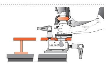
**15-14** When placing long horizontal boards in the rear clamp, make sure the rear end of the board is supported to prevent unnecessary racking of the jig.
