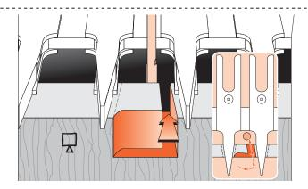
Rout through on the right side until the bit is clear of the workpiece. Move the bit to the left side and climb cut left to right.
