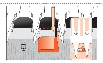
**15-3** Climb rout from left to right from the rear of the cut. **Take** care to control router.
