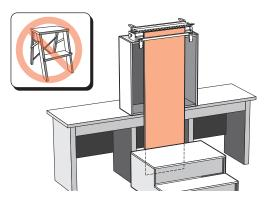
**15-13 General Hints** For routing long vertical boards it may be necessary to build a jig stand to mount securely on your bench. Make the stand and bench height combination sufficient to accept the board length you have in mind. The jig stand should be bolted securely to the bench. Build a stable platform to stand on as in the illustration. Do not use a set of steps; they're too unstable.
