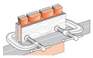
**15-11** A single scrap piece can be C-clamped on the back of halfblind tails, but make sure you protect the workpiece from the clamp pads. Note: There's no 100% solution to tearout. It's not the jig's fault, just something that happens when machining, sawing and even chiseling wood. Important pieces fall off from where you least want them to.
