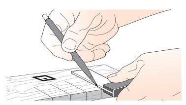
**13-8** On the test slot board only, square the marks across the face.
