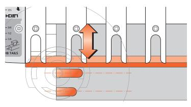
**13-13** Check to see if this short slot is centred on the pencil line. If not, adjust the finger assembly in or out and re-test on the other lines as necessary until the slot is centred. Lock the finger assembly in this position and record the setting for future reference.
