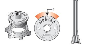
**13-4** Turn the e7-Bush to "5" and use the No. 120-8, ½"x 14° bit for sliding dovetails. This e7-Bush setting will allow for fine fit adjustment later.
