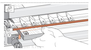
**13-10** Position and clamp the test board so that one of the edge marks is in line with the *outside edge* of the vertical board ③.
