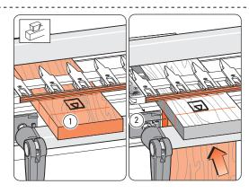
**13-9** Mount the test slot board in the rear clamp, markings up ①. Mount a ¾"[20mm] thick ② square-ended board vertically in the front clamp against the side stop, with the top edge butting the underside of the test board (yes, the ¾"[20mm] thickness is important).
