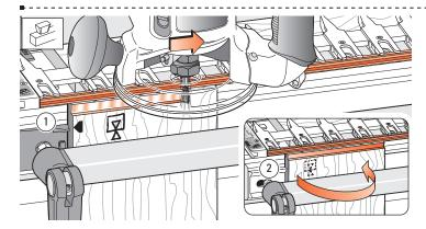
**13-3** Across the top ends of vertical boards to cut the tails. First rout one side ①...
