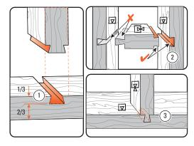
**13-5** On a full width joint, *the slot depth-of-cut should be no more than* 1/3 the board thickness ①. If the tail board is a load-bearing horizontal member (e.g., bookshelf or step), make the tail fairly thick for good tail neck strength ②. Shorter sliding dovetails for less structural demand may be slightly deeper, with narrower profiles, especially if appearance is important ③ (e.g., where narrow rails join wider boards).
