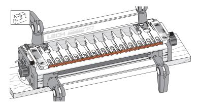
**13-1** With the finger assembly in the HB TAILS mode, the cross cut fence fits into the recesses in the ends of the tail guides to allow routing of sliding dovetails.
