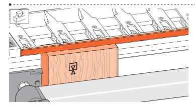
**13-15** Replace the spacer board in the rear clamp, and with the finger assembly on the spacer board, mount a test tail board vertically in the front clamp, **flush under the guidefingers**. Either side can face out  $\Box$ .
