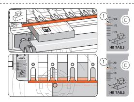
**13-11** With the finger assembly (including the cross cut fence) on the support brackets in the HB TAILS mode, set the scale to %6"[14mm] ①. The routed slot will be close to centred on the slot line. *Make sure the finger assembly is level and sitting flush on top of the board.*
