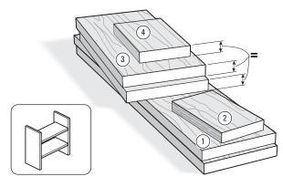
**13-6** Use  $\sqrt[3]{4}$ "x5 $\sqrt[4]{2}$ "[20x140mm] softwood to make two slot boards ①, plus one narrow test slot board ②, two tail boards ③ and one narrow test tail board ④. The tail boards ③ and test tail board ④ must be exactly the same thickness. This will make two uprights and two shelves.
