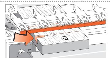
**13-12** Adjust the bit so the cut depth is about 5/16" [8mm]. Rout from left to right maintaining light inward pressure of the guidebush on the fence. Rout in only about 1"[25mm] and back out again.
