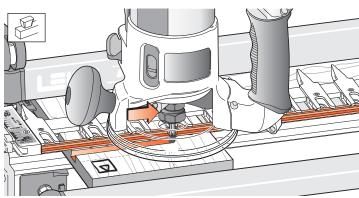
**13-2** Using the cross cut fence as a guide surface for the guidebush, you can make lateral router cuts across the faces of horizontal boards (dovetail *slots*), and...
