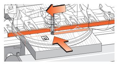
13-25 Dovetail slots preferably are routed from left to right because the bit's clockwise rotation pulls the guidebush against the fence. However; as when routing close to both ends of a board, it may be necessary to rout slots from right to left. Bit rotation will tend to pull the router away from the fence. Feed slower and maintain constant guidebush pressure against the fence.
