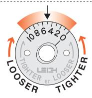
**13-21** Note: the e7-Bush fit adjustment for sliding dovetails works reverse to normal. Fit adjustments are made by adjusting the tail size only, not the socket. The e7-Bush is turned down to a lower number for a tighter fit, and up to a higher number for a looser fit. Each increment changes the glue line fit by 0.001"[0,025mm] When the fit is satisfactory, rout one end of a project tail board and test again. If the fit is good, rout all tail board ends.
