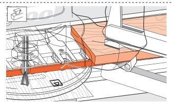
**13-24** Or lightly clamp (with a soft-jawed clamp) a short board to the finger assembly to act as a router stop.
