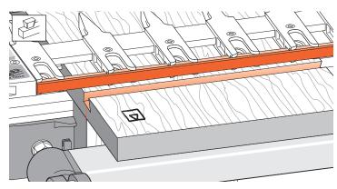
**13-14** Now rout sliding dovetail slots in the two main slot boards with the boards in the horizontal position in the rear clamp, slot side, that is inside face  $\square$  up.
