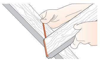
**13-19** Test the joint for fit. The tail should be too big. If it is too small, adjust the finger assembly outward by at least half the difference and rout another test tail on the other end of this test board.
