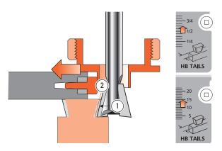
**13-20** If the tail is too wide ① move the finger assembly in toward the jig by half the amount the tail is too wide ②. Rout the same test board again. Adjust and re-test until fit is slightly loose or slightly tight.
