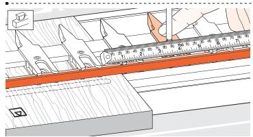
**13-23** Measure the same distance from where you want the slot stopped to a position on the finger assembly. Move a guidefinger to that point and mark the guidefinger with a felt pen as a visual router stop mark...
