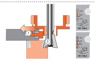
**13-16** The HB TAILS scale is not designed for this mode, but it does allow you to make quick adjustments for tail size and joint fit on sliding dovetails.
