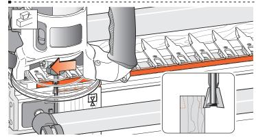
13-17 Rout one side of the test tail board.
