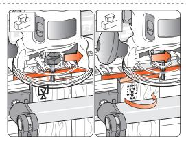
**13-18** Finish left to right, with the guidebush touching the fence. Turn the test tail board around in the jig and rout the other side in the same manner.
