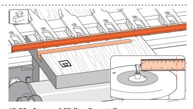
**13-22 Stopped Sliding Dovetails** If a stopped sliding dovetail is called for...
