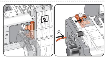
**10-8** The Spacer in the #1 position, slipped into the left-hand front side stop ① correctly offsets drawer sides ② from drawer fronts ③. The Spacer stays in place for the complete procedure. The Stop Rod stores here ④ and the Spacer here ⑤.
