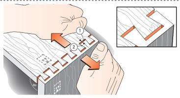
**10-19** Remove the boards and test the joint for fit. If the joint is **loose**, as shown here, **lower** the bit by the same amount as the gap at the bottom of the pins ① when the pins are pulled against the socket sides ②. If the joint is too **tight**, **raise** the bit slightly. Test again. You cannot rout the same board ends again with a dovetail bit, so use two fresh ends for each test.
