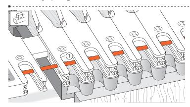
**10-7** Superjig features two novel innovations. A Stop Rod inserted through the fingers ① limits router travel to allow the deep tail socket guides to function as a simple shallow fixed comb.
