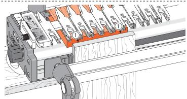
**10-10** Slip the Spacer onto the left hand front side stop ①, *note: No 1 to the top.* With the finger assembly raised in the HB Tails mode, clamp a drawer side in the front left side, against the Spacer and the top end edge slightly above the jig body top.
