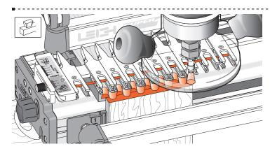
**10-18** Now rout in and out from left to right. Follow the guides into each finger opening to touch the stop rod. The pins, tails and sockets are formed simultaneously.
