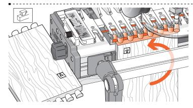
**10-24** To make a box, repeat the procedure four times, ensuring that the drawer fronts, rears and sides are all rotated correctly in the jig, keeping the inside face **□** of the boards away from the jig.
