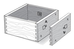
**10-25** Assemble the drawer. As with through dovetails, it doesn't matter which edge of any of the boards are at the top or bottom, the drawer will still fit together e.g. pin board "A" can be up either way.
