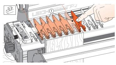
**10-15** Slide across enough guide fingers to cover the **drawer front width**. Position fingers tight together and center the group of fingers on the board ①.
