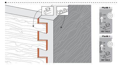
**10-22** If the tails stand out from the pins, set the HB TAILS scale **away from the operator** by half the amount required.
