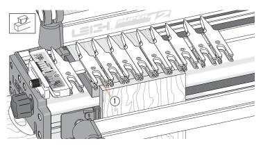
**10-14** With the scale set on ½"[12,7mm], raise the finger assembly about ½6"[2mm] above the drawer front ①. The scale is always set on the 1/2" mark when using the stop rod. *See 10-26 for Drawer Sides (Tail Boards) thicker than 5/8"*.
