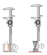
**10-4** Cumulative plus/minus tolerances in routers, bits and guidebushes, make it impossible to state exact bit depth for first-time precision fit. All dovetail jigs require trial and error tests to attain a fine fitting joint. The good news; we give a starting depth for each bit. Test and measure the successful 'Best fit' depth of cut ① or bit projection ② and record for future first-time fits.
