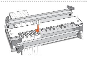
**10-6** This is a typical fixed template comb type jig. The comb depth ① is usually dimensioned to suit the most popular drawer side thickness of ½"[12,7mm].
