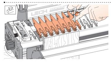
**10-16** Tighten the finger's screws. Move any spare fingers so that they will support the router and **tighten all loose fingers**. Lower the assembly **flat onto the two work pieces**.
