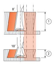
**10-3 Bit Angle and Depth of Cut.** Half-blind pins and tails are routed with the **same** dovetail bit, the **same** guidebush, and the **same** depth of cut. A different depth of cut requires a different angled bit. Leigh offers five different angled dovetail bits for a range of cut depths. A lesser angle, say 8°, for a deeper cut ①; a greater angle, say 18°, for a shallower cut ②.
