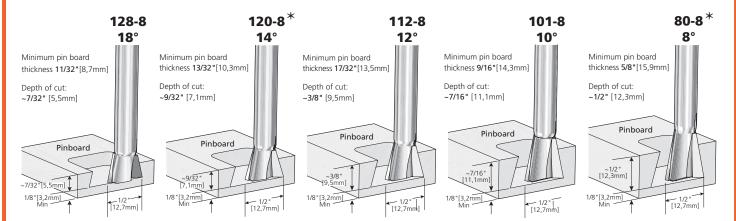
Note: Add at least ½" [3,2mm] to the depth of cut for board thickness. ★ Included with jig. ~ Symbol for "Approximately"
