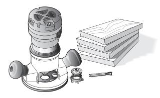
**10-5 Routing a Test Joint** You need a router, the e7-Bush set at No.10, the 80-8 ½"[12,7mm] 8° dovetail bit, two ¾"[19mm] thick pin boards and two ½" thick tail boards. The No.80-8 bit routs at a shallower ~½"[13mm] depth on single pass dovetails than on regular variably spaced joints. For this test, start with the No.80-8 bit projecting 1"[26mm] from the router base.
