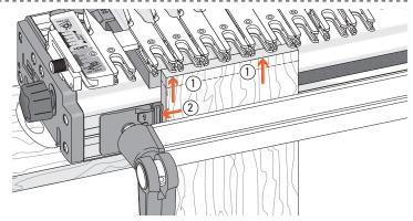
**10-13** Re-set the drawer side in the front clamp so that its top edge touches the guide fingers and is **perfectly flush** with the top face of the drawer front ① and the left edge is against the Spacer ②.
