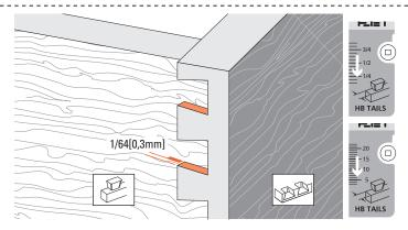
**10-23** If the tails fit in too far past the pins ends, set the HB TAILS scale **toward the operator** by half the amount required.
