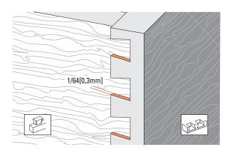
**10-21** When you have the proper tightness of fit, check the flushness. The tails should be under flush to the pins by *no more than 1/64"[0,3mm] to allow for cleanup (exaggerated here)*. Any concentricity errors in the collet and guidebush on different routers will affect this tolerance.
