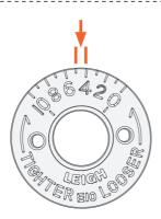
**3-7** One increment of the eBush changes the joint glue line by 0.002"[0.05mm]. Half an increment changes the fit by an incredible 0.001"[0.025mm]. A perfect fit will be established with one or two test cuts.
