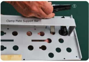
Insert the second clamp in the inner clamp hole from **ABOVE** the clamp plate support bar.
