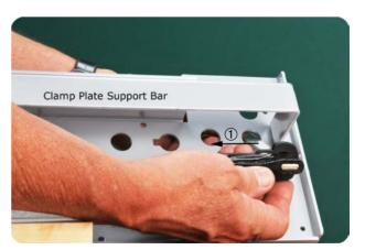
Insert the first clamp from **UNDER** the clamp plate support bar and into the outside clamp hole. **Note:** The tip of the clamp must point towards the center of the jig. ①
