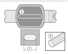
**6-13** For mortises and tenons shorter than the guide, reverse the calculation: Guide, minus Joint, divided by 2.
