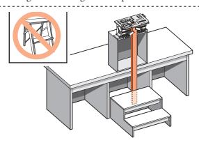
**6-18** To rout long vertical boards you could build a jig stand to mount on your bench. Make the stand/bench combination high enough to accept the desired board length. *Bolt securely to the bench.* Make a stable platform as shown here to stand on. **Don't use a folding step, these are unstable.** Other novel solutions: holes in (suspended) floor; jig bolted to deck or mezzanine railing; wall brackets.
