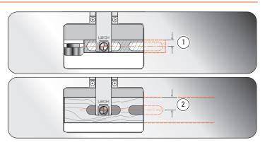
**6-2** Single or double (in-line) mortise and tenons are straight forward. Simply mount and sight and rout all the tenons as shown before ①, then mount and re-sight the mortises at the desired front-back position before routing ②.
