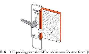
and if required frequently, should have sandpaper glued onto its outer surface for secure workpiece clamping ②.
