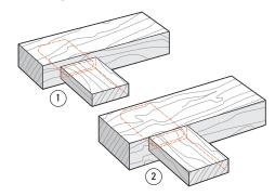
**6-1** So far we have only illustrated joints where the mortise and tenon workpieces are the same thickness. There will be numerous times when this is not the case, as in where the tenon piece is thinner and centered on the mortise board ①, and where the tenon piece is deliberately off-center on the mortise piece ②.
