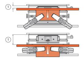
**6-20** Use the Leigh clamps to secure the bracket to the FMT Pro clamp face and adjust the distance below the table to slightly greater than the mortise piece thickness ①.
