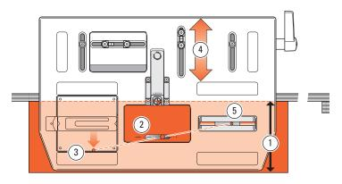
6-22 Mortises in center of boards 45/8" to 61/2" [115 to **165mm]** ①: Mark mortise center on a test board ②. Using the guide recess front edge as mortise guide 3, adjust the table to center the mortise 4. Control mortise length with 3/16" [5mm] dowel pieces in the pin track (5) (see 6-16). Note: This is not a standard Leigh solution, but we thought it would solve this rare challenge.
