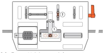
**6-6 Tenons** Mark the center as before. Position and sight the tenon ①, and lock the table. Set the  ${}^{\circ}$ **FB** stops against the post ②.
