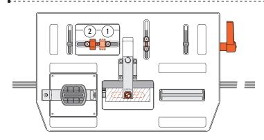
**6-7** Set the <code>qpLR</code> stops one at a time with the small block between the stops and post ①②. This ensures that the table movement is centered about the joint center-mark on the stock. Remove the block, **but save it**.
