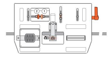
**6-14 Tenons** Setting the block and limit stops for the shorter tenons procedure ①② is exactly the same as for longer tenons setup, except when you come to rout.
