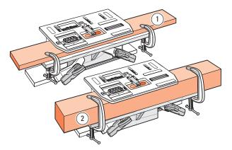
**6-21** Use C-clamps to hold the workpiece onto the bracket, with the workpiece rear edge touching the clamp plate. Now raise the bracket so the workpiece touches the underside of the table. Re-secure with the Leigh Clamps. The widest board in which a mortise may be centered is 45/8" [115mm] ①. The thickest capacity is 4"[100mm] ②.
