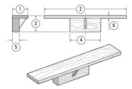
**6-19** Make this bracket to mount and mortise a wide board face, clamp pieces greater than Leigh Clamp 3" capacity, and center mortises on boards up to 45/8"[115mm] wide or even 63/8"[162mm].
