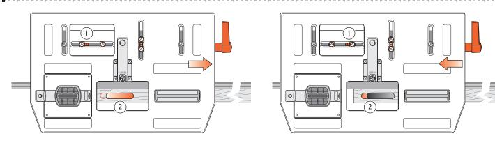
**6-11** Move the table **right** to the stop ①. Rout the **right-hand** end of the mortise ②, using the full length of the mortise guide.
