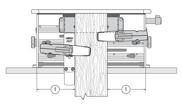
**5-4** Set the sidestop fence so that the tenon piece is clamped approximately centrally on the clamp plate ①.
