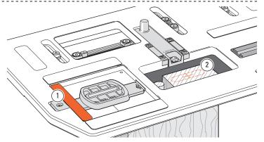
**5-8** Move the table right and lock. Lift the left end of the (stationary) router and move the "tenon guard" left ①. Rout the right hand tenon ②. Repeat as required for all tenon ends, moving the table "guard" piece only once for each pair. Leave the table to the right. Remove and save the guard. Note: If you change the plunge height between tenons, there's the chance of having a step in the shoulder. We recommend leaving the bit plunged.
