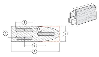
**5-34** Because of safety considerations it is only practical to rout triple joints with  $\frac{3}{8}$  bits and guides or smaller.
