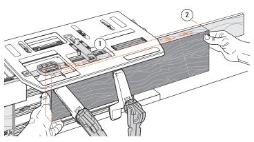
**5-9** Extend the sight. Position and clamp the mortise piece so the right hand mortise of the first pair is centered under the sight ①. Either mark an outrigger or set a stop block for successive mortise pieces ②. Rout the right hand mortise. Note: Outriggers are referenced in Step 3-19.
