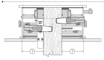
**5-36 Tenons** Center (approximately) and clamp the tenon workpiece on the clamp plate ① and set the side-stop fence.
