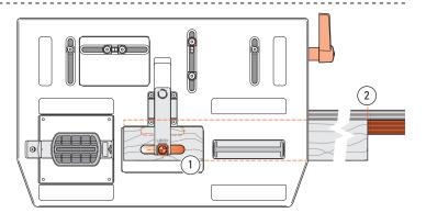
**5-19 Mortises** Extend the sight. Position and clamp the mortise piece so the left end front mortise is centered under the sight ①. Either mark the right hand outrigger or set a stop block for successive mortise pieces ②. Rout the front mortise.
