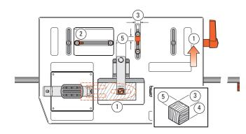
**5-39** Release the table clamp and move the table to sight the third (single) tenon ①. Lock the table.
