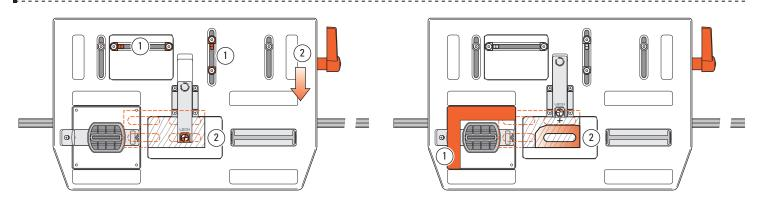
**5-28** All four stops are now set ① and provided you have symmetrically marked out the joint, moving the table to the front right-hand tenon, the sight should automatically align with that mark ②. If it does not, do not change anything. Just check the other three positions; the actual joint will be symmetrical.
