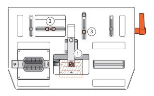
**5-15** Unlock the table, sight the rear tenon center and lock the table ①. Set and lock both ap LR limit stops against their stop post ②. Set and lock the front against its stop post ③.
