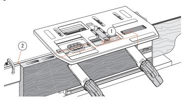
**5-11** Extend the sight and unclamp. Sight the left of the other pair of mortise positions ① and re-clamp. To avoid re-sighting each board, mark the left hand outrigger or set a stop at the workpiece end ②. Rout the mortise, then move the table and rout the right hand mortise. The table limit stops and outrigger marks (or stops) are now set for successive workpiece mortising.
