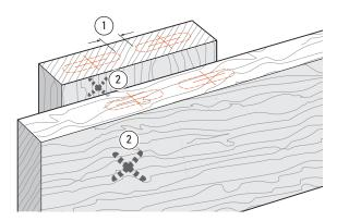
**5-3** Mark the two mortise and tenon centers, taking care to allow space between the joints ① at least equal to the tenon bit diameter. Mark the faces that go against the clamp plate 2.
