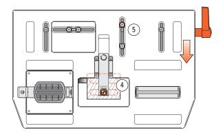
**5-16** Unlock the table and sight the front tenon ④ and lock the table. **Set and lock the rear** �**FB** stop against its post ⑤. Unlock the table and move the table front to back against the stops to double-check the tenon sighting.
