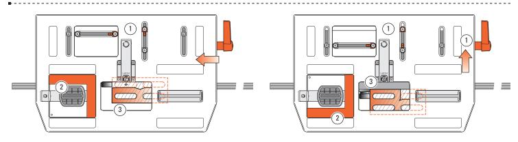
**5-30** Move the table to the front left against the stops and lock 1. With the "guard" at the rear-right 2, rout the front-left tenon 3.
