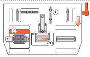
**5-18** Move the table forward and lock ①. Lift the left end of the router and move the "tenon guard" to the rear ②. Rout the front tenon ③. Repeat as required for all tenon ends, moving the table and guard piece only once for each pair. **Leave the table forward.** Note: By using two or three left-right table positions, (in addition to the front-back positions), the workpiece width and tenon width may be increased to the maximum (see Chapter 6, Longer and Shorter Joints).
