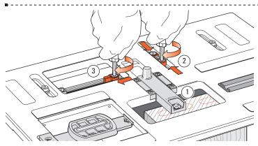
Sight the left hand tenon and lock the table ①. Set and lock both **FB** limit stops against their stop post ②. Set and lock only the right hand ap LR limit stop against its post 3.
