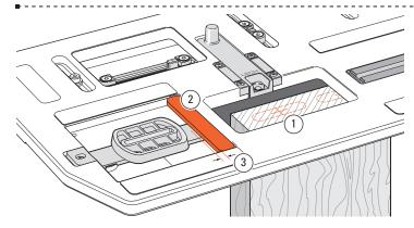
**5-7** Move the table left and lock. **Do not rout yet.** While with practise it is fairly easy to avoid routing "into" the right tenon while routing the left ①, we recommend that beginners use a small shop-made "guard" to prevent this 2. Use 1/4" [6mm] thick MDF or plywood. Allow a 3/16" [5mm] gap between the end of the guide and guard 3. Rout the left tenon.
