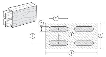
**5-22** The **maximum** dimensions for quadruple joints are: Tenon Workpiece ①: 3" x 5½"[70 x 140mm]
