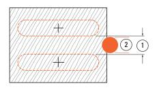
**5-13** Mark the two tenon centers taking care to allow space between the two joints ① at least slightly greater than the tenon bit diameter ②.
