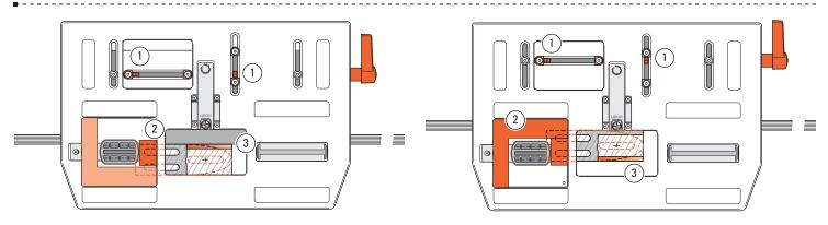
**5-42** So to reduce the thickness, move the table right and rearward against the stops ① as if to rout a quadruple tenon. Then add a small "guard" piece 2 to the L-shaped guard in the guide recess. Now rout away part of the workpiece 3.
