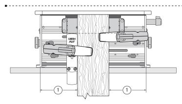
**5-24** Center (approximately) ① and clamp the tenon board on the clamp plate and set the side stop fence. Note: If the tenon board does not touch the underside of the table, extend the sight to stop the board.
