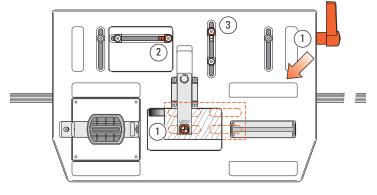
**5-25** Extend the sight, release the table clamp and move the table to sight the **left hand front** tenon ①.
