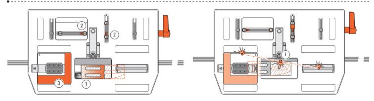
**5-40** Rout the left pair of tenons in the same way as for the quadruple tenons ① (see 5-30 and 5-31), using the Limit Stops ② and an L-shaped guard 3 in the guard recess to prevent accidental routing of adjacent tenons.
