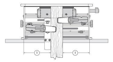
**5-14** Approximately center the table left to right and lock ①. Extend the sight. Clamp the tenon piece against the sidestop fence, the tenon piece lightly touching the underside of the sight.
