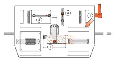
**5-37** Extend the sight, release the table clamp and sight the front tenon of the pair ①. Lock the table, move the right hand ap LR limit stop to the post and lock ②. Move the back **\$FB** limit stop to the post and lock ③.
