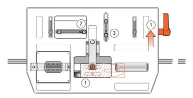
**5-38** Release the table clamp and sight the rear tenon of the pair ①, making sure that the right-hand ap LR stop is against its post 2.
