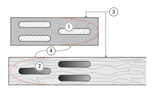
**5-46** Remember, mortises are routed the opposite way around to their matching tenon, e.g. in this illustration the single tenon is to the right ①, single mortise to the left ②. Keeping the reference faces together on the finished joint will ensure that the mortises and tenons will align ③. It's much easier to clamp square section workpieces so do not do any shaping of workpieces until after the joints are routed ④.
