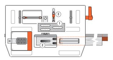
**5-44** Release the table clamp. With the table to the right, against the <sup>ap</sup> **LR** stop, put the small block between the rear **BB** stop and its post ①. You must always use the same limit stop for all other third tenons and mortises. Using a guard to avoid routing, into the other two tenons ②, rout the rest of the third tenon ③.
