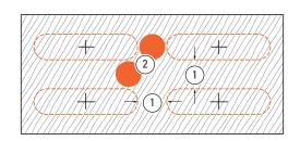
**5-23 Tenons** Mark the four tenon and mortise centers to suit your layout. Take care to leave a space between tenons ① at least slightly greater than the tenon bit diameter ②.
