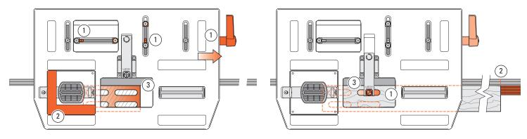
**5-32** Move the table to the rear right against the stops and lock ①. Move the "guard" to the front-left ②. Rout the rear-right tenon ③. Rout all other tenon ends required. Leave the table to the rear-right.
