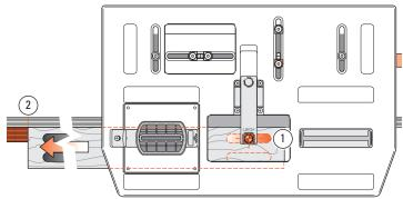
**5-21** Extend the sight, unclamp and move the mortise board left so that the rear mortise of the pair at the right end of the piece is centered under the sight ① and re-clamp. Mark the left hand outrigger or set a stop ② adjacent to that end of the workpiece. Rout first the rear mortise at this (right-hand) end, then move the table and rout the front mortise. The outrigger marks or stops are now set up for successive workpiece mortising.
