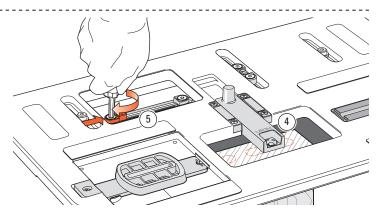
**5-6** Unlock the table and sight the right-hand tenon ④ and lock the table. Set and lock the left hand ap LR limit stop against the post 5.
