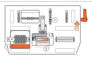
**5-17** Move the table to the rear against the stop and lock ①. Do not rout yet. While with practise it is fairly easy to avoid routing into the front tenon ② while routing the rear, we recommend that beginners use a simple shop-made "guard" ③ to prevent this. Use ½"[6mm] thick MDF or plywood. Allow a ¾16"[5mm] gap ④ between the side of the guide and guard. Rout the rear tenon ⑤.
