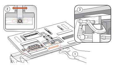
**4-16** Extend the sight. With the marked side of the mortise piece toward the clamp plate, either move the board left and right ① to align the cross with the sight and clamp in place; or clamp in place first and move the table to align the sight ②. Remember, you previously set the <code>%FB</code> limit stops to allow only left/right movement. For routing very small pieces ③, see 3-16.
