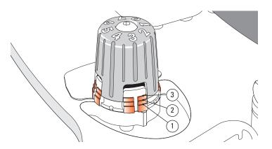
**4-10** Check that the left hand knob is two turns up. From this setting the actual fit setting will be established by trial and error and the result recorded for each guide/bit combination.
