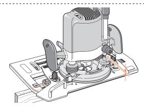
**4-17** Place the router/Sub-Base assembly on the jig, the left hand guide pin in the mortise slot part of the guide. Now raise the plunge stop rod slightly, say ½32-½16"[1-1,5mm] to allow the mortise to be routed slightly deeper than the tenon to ensure perfect tenon shoulder flushness on the finished joint.
