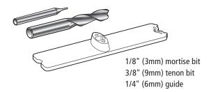
4-36 Example: 1/8" (3mm) Mortise & Tenon Joints with a 1/4" (6mm) Guide Using the two bits and guide shown above, you can rout a 1/8" (3mm) mortise and tenon. The resulting joint is 1/8" (3mm) smaller than the 1/4" guide size. Note: Any two bit diameters that add up to twice the guide size will produce a joint size of the smaller bit.
