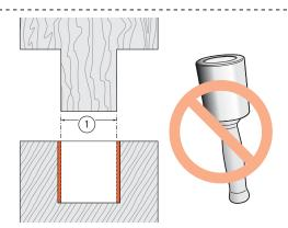
**4-25** Generally we have found the best fit differential to be 0.005"[0,13mm] "loose". Basically, the dry joint should "push" together fairly easily, but not fall apart under its own weight. If a mallet is needed, it's too tight.
