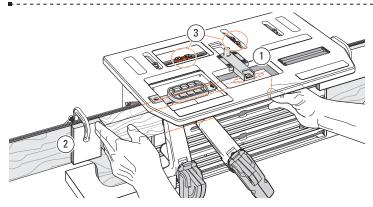
**4-29 Mortises:** Sight one mortise ① and set a stop block at the end of the mortise board ②. Set <code>apLR</code> limit stops and <code>\$FB</code> limit stops to prevent unintentional table movement ③.
