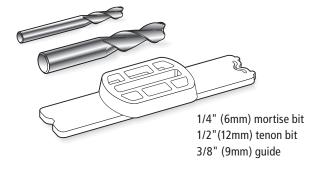
**4-34** Example: 1/4" (6mm) Mortise & Tenon Joints with a 3/8" (9mm) Guide Using the two bits and guide shown above, you can rout a 1/4" (6mm) mortise and tenon. The resulting joint is 1/8" (3mm) smaller than the 3/8" (9mm) guide size. Note: Any two bit diameters that add up to twice the guide size will produce a joint size of the smaller bit.
