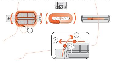
**4-14** Routing counter-clockwise, run the guide pin around the tenon guide surface. Make sure the pin contacts the entire outer surface ①. In these first test cuts, check the tenon for a completely smooth cut before removing the piece from the jig. Until you are confident with this procedure, we recommend as a final clean-up, you run the guide pin "off" of each guide "corner" ② in both directions ③.
