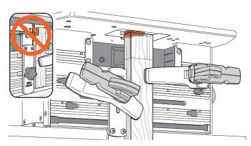
**4-4** Clamp the tenon piece with the end edge lightly touching the underside of the sight. Its side edge should touch the previously set side stop fence, with the marked side toward the clamp
