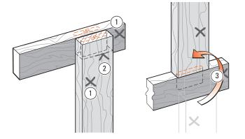
**4-2** In almost all cases, it is critical to have the same side of workpieces reference against the clamp plate for each tenon and mortise. So mark one side of each workpiece to reference "this side toward the clamp plate" ①, or "away from" if you prefer. Make a pencil mark ② to the required shoulder depth on the tenon workpiece. When the joint is cut, the tenon piece is rotated 180° to assemble ③.
