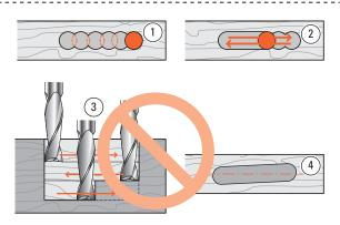
**4-18** The best way to rout mortises (parallel to workpiece) is plunge full depth, slightly overlapping holes ①, then clean out left-right-left at full depth of cut ②. **Do not rout left-right-left at progressively greater depths without plunging holes** ③ ... the bit's rotation will pull the bit off the intended mortise line with each pass ④ and the mortise may not be parallel to the workpiece.
