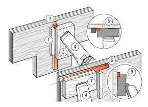
**4-40** To hold very small workpieces ②, make up a rabbeted holder ③ with the rabbet slightly shallower than the workpiece thickness, leaving a gap at ⑤ and ⑨. i.e. For Tenons: Side stop ① Tenon Piece ② Holder ③ Clamp ④ Gap ⑤. For Mortises: Mortise Piece ⑥, Holder ⑦, Clamp ④, Gap ⑨. ■
