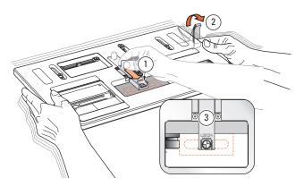
**4-3** If you have not yet mounted the side stop fence, do so now (see 3-13 to 3-15). Place it off center by about half the width of the tenon piece; either side, it doesn't matter. Pull the table sight forward to its stop ①. Release the table clamp ② and move the table to position the sight over the approximate tenon piece position 3. Lock the table. Always lock the table before positioning workpieces.
