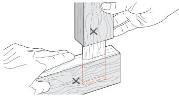
**4-20** Remove the mortise piece and test the tenon for fit and (keeping the marked faces adjacent) for flushness. If the face sides are not flush, check the straightness of the two parts. If they are straight, the clamp plate may not be vertically parallel to the bit. See Appendix II, Jig Adjustments, A2-1 through A2-3.
