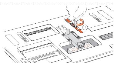
**4-6** Unlock the two **FB** front/back limit stops. Move both so they touch the Stop Post and tighten both stops ①. This prevents front-to-back movement of the table when later sighting the mortise. Retract the sight.
