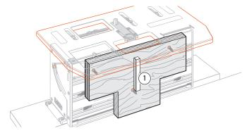
**4-39** For very small joints we recommend attaching a rigid piece of ply or MDF minimum <sup>3</sup>/<sub>4</sub>"[20mm] to the clamp plate, using the through screw holes in the plate. This should have its own mini side stop fence attached for tenons ①.
