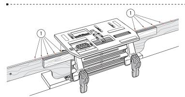
**4-31** Successive mortises in "ladder" type construction are quick to rout. Mark all mortises on only one piece (only one needs a front-to-back mark!). Sight the first mortise (cross) to set the table and mark the top of one outrigger in line with the workpiece end. Table locked, move the workpiece, sighting each successive mortise line, marking the outrigger(s). To rout, align the unmarked board ends with the outrigger marks ①.
