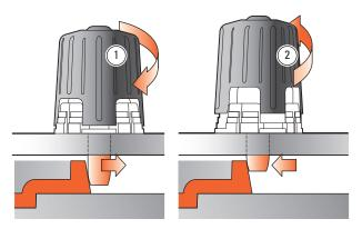
**4-21** If the joint is too loose, turn the guide pin down ①. If the joint is too tight, turn the guide pin up 2. For how much, see 4-22. Rout a complete new joint. Note: It's possible to adjust the guide pin and rout only one new mortise or tenon part and get a good fit, but on a project this would mean routing each part at different settings. Establish ideal pin height for both mortise and tenon at one pin setting.
