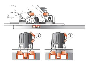
**4-9** Adjust the right hand guide pin. Grip the right hand pin knob and move the Sub-Base back and forth to feel the "free play" of the pin across the slot width ①. Turn the knob down ¼ of a turn at a time, to feel the "play" diminish ②. When the "play" stops, turn the knob up ½ of a turn until the slightest play can be felt ③. The router/Sub-Base should slide freely left to right. If the right pin is a little "sticky", turn it up a bit more.
