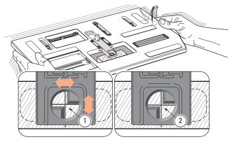
Release the table clamp and move the table until the sight opening is positioned equally around the cross lines on the workpiece. Lock the table. Because the human eye excels at comparisons, differences as small as 0.004" can be perceived in the space between the edges of the line and the triangles as shown here ①. You can readily center the sight using slight table movements until the spaces appear the same 2.
