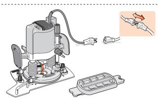
**Unplug the router.** Insert the selected guide to the guide recess and matching diameter bit to the router.
