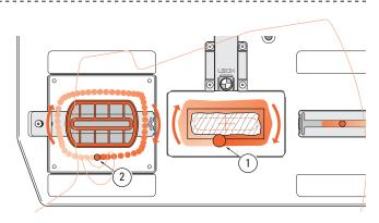
**4-12** Read all of the next three instructions before routing. With the guide pin in the near side of the guide recess, switch on the router power and with firm control, move it in until the bit lightly touches the tenon workpiece. Very carefully, with the bit very lightly engaging the wood surface, "climb rout" clockwise around the tenon piece ①. Maintain very light bit contact. Do not run the guide pin on the guide yet ②.
