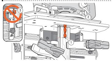
**4-11** Plunge the router so the tip of the bit is level with the pencil mark of the tenon shoulder and lock the plunge ①. Set the plunge depth stop rod to its stop ②. *Generally, tenons are routed in one depth setting, it is not necessary to make multiple passes at different depths of cut.* WARNING: Never rout tenons with the sidestop fence in the inverted position ③.
