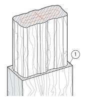
**4-13** Control the router firmly, the router is driven clockwise by the bit rotation. This first shallow climb cut will leave a small but clean shoulder ①.
