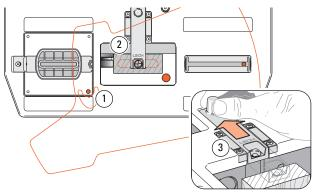
**4-28 Tenons** The router is "parked" with the guide pin in near front corner of recess ①. Extend sight and use only as a tenon stop ② when clamping successive (unmarked) tenon pieces against side stop. Retract sight ③ and rout any number of tenons without removing router. **Note:** If you forget to retract the sight, the Sub-Base will push it out of the way as you move it rearward, but we do not recommend this.
