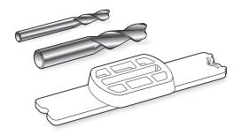
**4-33 Two Bit Combination** If you want to rout many ¼"[6mm] mortises and tenons, the tenons can be routed much more quickly with a ½"[12mm] bit\*. The Guide and Bit Selection charts in Appendix I show how different bit combinations can crank out such extraordinary joints just as quickly and precisely as larger ones, and with adjustable joint tightness.
