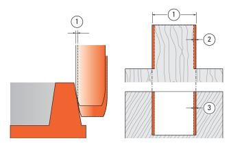
**4-22** How much adjustment is required? One eighth of a turn of the guidepin knob will change the joint glue-line fit by 0.001"[0,025mm] ①, i.e. turn one-eighth up; the bit will reduce the tenon thickness by 0.001"[0,025mm] (half of that per side ②) and increase the mortise width by the same amount 3. Dimensions and angles shown here are exaggerated.
