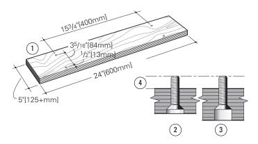
**1-1 Mounting the FMT Pro:** Prepare a flat board at least  $\frac{3}{4}$ "[20mm] thick, a minimum of 24"x5"[600x125mm]. Drill four  $\frac{3}{2}$ "[7mm] holes on  $15\frac{3}{4}$ "x3 $\frac{5}{16}$ "[400x84mm] centers,  $\frac{1}{2}$ "[13mm] in from the front edge of the board ①. Countersink ②, or counter-bore ③ if board is thicker, the underside so that the four  $\frac{1}{4}$ —20 x 1" long machine screws will project above the top surface by  $\frac{3}{8}$ "[9,5mm] ④.
