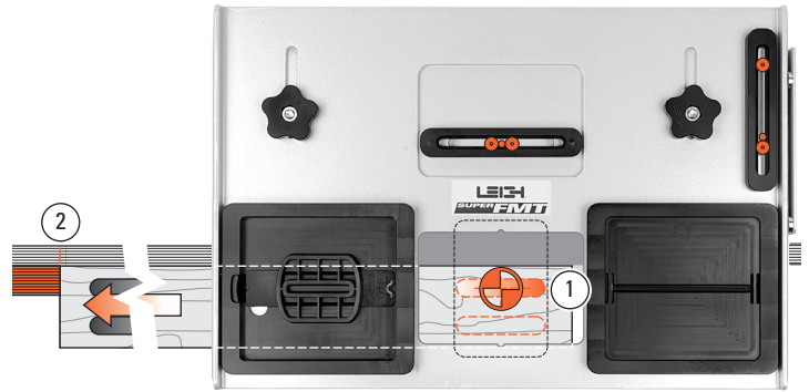
5-21 Replace the sight, unclamp and move the mortise board left so that the rear mortise of the pair at the right end of the piece is centered under the sight ①, and re-clamp. Mark the left hand outrigger or set a stop ② adjacent to that end of the workpiece. Rout first the rear mortise at this (right hand) end, then move the table and rout the front mortise. The outrigger marks or stops are now set up for successive workpiece mortising. ■
