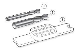
**4-33** For example, if you want to rout many  $\frac{1}{4}$ "[6mm] mortises and tenons, the tenons can be much more speedily routed with a  $\frac{1}{2}$ "[10mm] bit. Here's how.
