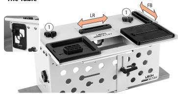
**3-11** The table is clamped in any desired position by the Table Clamp Knobs ①. Loosening the knobs slightly releases the table, which can then be moved in any direction to any position within its range.
