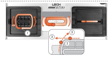
**4-14** Routing counterclockwise, run the guide pin around the tenon guide surface. Make sure the pin contacts the entire outer surface ①. In these first test cuts, check the tenon for a completely smooth cut before removing the piece from the jig. Until you are confident with this procedure, as a final cleanup we recommend you run the guide pin "off" of each guide "corner" ② in both directions ③.
