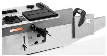
**4-30** Sight the second mortise by moving the mortise piece (not the table), and set the second stop block ①. Rout any number of successive (unmarked) mortises without removing the router from the table.
