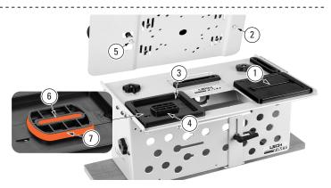
**3-14** To the right front is the right hand "Guide Pin Track" ①. The right hand router sub-base Guide Pin ② runs in this track in all routing operations. To the left front is the Guide Recess ③, in which all Joint Guides ④ are placed. The left hand router sub-base Guide Pin ⑤ runs in the guide slot ⑥ for routing mortises, or around the outside of the Guide ⑦, for routing tenons.
