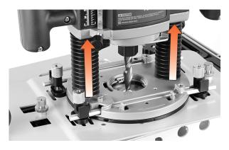
**3-34** Always raise the plunge router mechanism before removing the router assembly from the jig.
