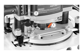
**3-31** Make sure the router collet does not contact the Super FMT sub-base at full plunge cuts ①. Set the router plunge stop rod as necessary to prevent this ②.
