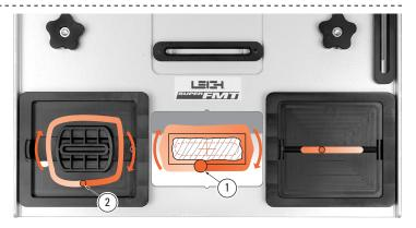
**4-12** Read **4-12** through **4-14** before routing. With guide pin in near side of guide recess, switch on router power and with firm control, move it in until the bit lightly touches the tenon workpiece. Very carefully, with the bit very lightly engaging the wood surface, "climb rout" clockwise around the tenon piece ①. Maintain very light bit contact. **Do not run guide pin on guide yet** ②.
