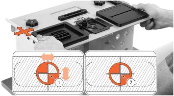
**4-5** Loosen the table knobs and move the table until the sight opening is positioned equally around the layout marks on the workpiece. Lock the table. Because the human eye excels at comparisons, differences as small as .004 can be perceived in the space between the edges of the line and the triangles as shown here ①. You can readily center the sight using slight table movements until the spaces appear the same ②.
