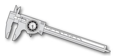
**4-24** If you have a dial or digital calliper (every shop should have one) you can literally measure the tenon and mortise and adjust accordingly. Every ~0.002"[0,05mm] of difference in mortise to tenon size (say ~.001"[.025mm] on the glue line) should require ½ of a turn; down to tighten, up to loosen.
