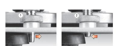
**4-21** Joint fit is adjusted with the left hand guide pin only. If the joint is too loose, turn the guide pin down ①. If the joint is too tight, turn the guide pin up ②. For how much, see 4-22. Guide pin changes affect the mortise and tenon, so rout a complete new joint. Establish ideal pin height for both mortise and tenon at one pin setting.
