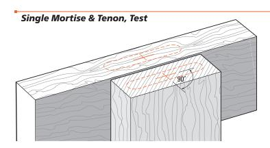
**4-1** Let's make a plain single mortise and tenon. Using a fine pencil, mark a cross at the center of the required tenon and mortise positions, the cross lines along and across the axis lines of the joint, at 90° to each other. Mark the mortise several inches[10cm] or so away from the end.
