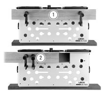
**4-15** Remove the router and tenon workpiece from the jig. Position the two clamps so the mortise piece can be positioned for secure holding. Clamp to either both sides of the bit opening ① or to one side ②. Note: Leaving a "horn" on the ends of mortise pieces as in ① not only makes for easy clamping, the horns will be an aid in assembly gluing and clamping later. Refer to 3-3.
