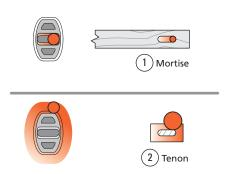
**4-35** Using a small guide, combined with an even smaller mortise bit and larger tenon bit gives the Super FMT an additional unique ability to rout joints smaller than the smallest (¼"[6mm]) guide. For example, take a ¼"[6mm] guide and **step up** by ½"[3mm] to ¾"[10mm] diameter on the tenon bit...and **step down** the same amount for mortise bit to get ½"[3mm] mortise and tenons...**all with adjustable joint tightness.**
