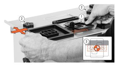
**4-3** If you have not yet mounted the sidestop fence, do so now (see 3-7). Place it off center either side, it doesn't matter which. Fit the table sight in the bit opening ①. Loosen the table knobs ② and move the table to position the sight over the approximate tenon piece position ③. Lock the table knobs. Always lock the table before positioning workpieces.
