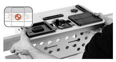
**4-16** Fit the sight and remove the sidestop fence if it is in the way. With the marked side of the mortise piece toward the clamp plate, either move the board left and right to align the cross with the sight and clamp in place, or clamp in place first and move the table to align the sight. Remember, you previously set the **FB** limit stops to allow only left/right movement.
