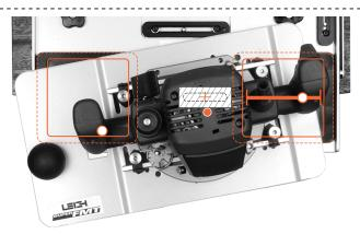
4-8 Make sure the two guide pins are turned up approximately two-and-a-half turns from the lowest position to avoid the end of the guide pin contacting the bottom of the guide pin track and guide recess! Place the router on the jig table, the right-hand guide pin in the right side track, the left-hand guide pin in the near side of the guide recess.
