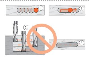
**4-18** The best way to rout mortises (parallel to workpiece) is to plunge slightly overlapping holes to full depth ①, and then clean out left-right-left at full depth of cut 2. Do not rout left-right-left at progressively greater depths without plunging holes 3...the bit's rotation will pull the bit off the intended mortise line with each pass 4 and the mortise may not be parallel to the workpiece.
