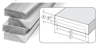
**3-38** You will want to test the jig, so prepare some stock with a thickness **A** about 2.5 to 3 times the bit diameter **B**.
