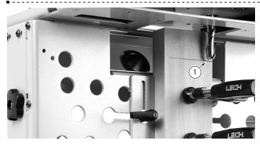
**4-11** Plunge the router so the tip of the bit is level with the pencil mark of the tenon shoulder ①, and lock the plunge. Set the plunge depth stop rod to its stop. Tenons are routed in one depth setting; it is not necessary to make multiple passes at different depths of cut.
