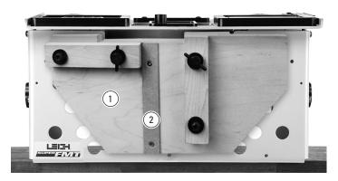
**4-37** For very small joints we recommend attaching a rigid piece of ply or MDF ① minimum ¾"[20mm] to the clamp plate, using the through screw holes in the plate. This should have its own mini sidestop fence attached for tenons ②.
