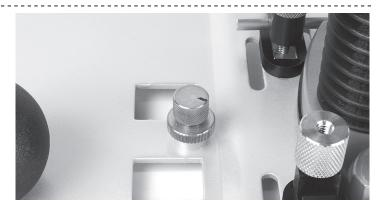
**4-26** Once you've established the guide pin setting for a specific bit/guide combination, record the setting on the following page. For example:  $\frac{5}{16}$ "x1 $\frac{1}{2}$ "[8x35mm] "up  $\frac{1}{4}$  turns". Using the same bit and guide next time, use the recorded setting for a good fit first time. Note: Different wood species may require slightly different settings.
