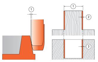
**4-22** How much adjustment is required?  $\frac{1}{8}$  of a turn of the guide pin knob will change the joint glue-line fit by 0.001"[0.025mm] ①, i.e. turn  $\frac{1}{8}$  up; the bit will reduce the tenon thickness by -0.001"[0.025mm] (half of that per side ②) and increase the mortise width by the same amount ③. Dimensions and angles shown here are exaggerated.
