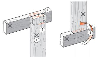
**4-2** In almost all cases, it is critical to have the same side of workpieces reference against the clamp plate for each tenon and mortise. So mark one side of each workpiece to reference "this side toward the clamp plate" ①, or "away from" if you prefer. Make a pencil mark ② to the required shoulder depth on the tenon workpiece. When the joint is cut, the tenon piece is rotated 180° to assemble ③.
