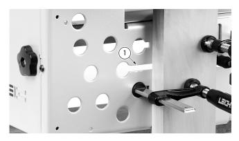
**3-5** The clamp plate holes allow for full clamping coverage. The two long keyholes ① are for the sidestop fence, but these holes (not the slots) may be used for clamping if required.
