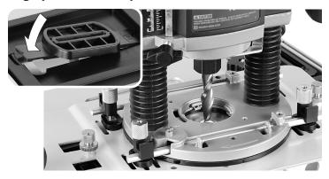
**3-20** Select a guide and bit. Snap the guide into the guide recess and install the bit in the router.
