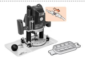
**4-7** Unplug the router. Insert the selected guide into the guide recess and matching diameter bit into to the router.
