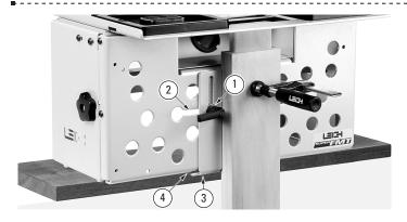
**3-7** The sidestop fence is attached by a single index lever ① and carriage bolt inserted through one of the two 'keyhole' slots ②. Most tenon pieces are routed vertically, and for that purpose the bottom of the fence ③ acts as a T-square against the bottom edge of the clamp plate ④. See Appendix II (A2-5), for sidestop squareness adjustment.
