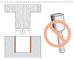
**4-25** Generally we have found the best fit differential to be 0.005"[0,13mm] "loose". Basically, the dry joint should "push" together fairly easily, but not fall apart under its own weight. If a mallet is needed, it's too tight.
