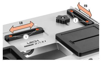
**3-12** Adjustable Limit Stops ① are used to limit or prevent table movement left to right (X-axis) and front to back (Y-axis), and to precisely align double and quadruple mortises and tenons (see Chapter 5). Use Limit stops when you see these icons:
