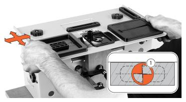
**3-23** The jig table is centered over the marked workpiece with the sight ①.
