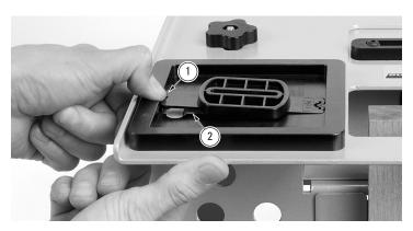
**3-18** To remove a Guide, pull back the latch ① and push through the hole from below with your fingertip ②.
