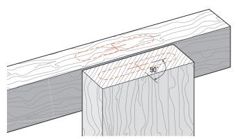
**3-21** The centers of a mortise and a tenon are marked with a cross.
