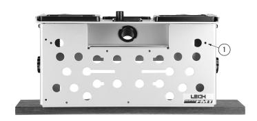
**3-6** The clamp plate is provided with seven small through-holes ①. If a facing board is required use No.8 or M4 wood screws (not supplied) from the rear. Alternatively the clamp plate holes could be marked onto a ply or MDF panel, bored through with a ¾" [20mm] Forstner bit and attached with a pair of optional Leigh F-Clamps.
