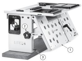
**3-1** The clamp plate ① is adjustable up to  $30^\circ$  from vertical and is held securely by two quadrant knobs ②. A set-screw ③ allows for positive return to  $90^\circ$ . To ensure flush and in-plane joints, it may be necessary to adjust the clamp plate angle. See Appendix II, Jig Adjustments.
