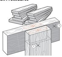
**4-27** When routing frame joints it is only necessary to mark and sight a single tenon and perhaps two mortises. Once the sidestop fence or outriggers are set and the table sighted for one joint, any number of similar joints may be routed without marking. We recommend marking the finished face which goes against the clamp plate (shown here from operator view) ①.
