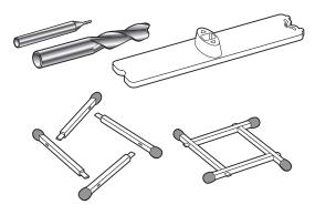
**4-36**  $1/32 \times 3/32$ " [0,8 x 2,4mm] mortises and tenons on this "match frame" were formed (with machine tool bits) on a 1/4" x 5/16" guide. The 1/5/32" tenon bit is 7/32" larger than 1/4". The 1/32" bit is 7/32" smaller than 1/4". A similar metric set: 6mm guide, 1mm mortise bit, and 11mm tenon bit produce 1mm joints. Machine tool bits as small as .010" with 1/4" shanks and similar metric bits are available from machine tool suppliers.
