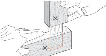
**4-20** Remove the mortise piece and keeping the marked faces adjacent, test the tenon for fit and flushness. If the face sides are not flush, check the straightness of the two parts. If they are straight, the clamp plate may not be vertically parallel to the bit. See Appendix II, Jig Adjustments, A2-1 through A2-3.
