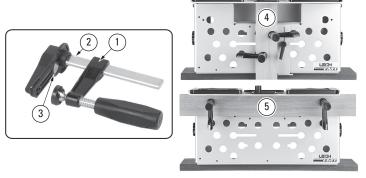
**3-2** The two F-Clamps have a capacity from zero to 3"[76mm]. The threaded clamp arm ①, is removable and the clamp bar ② is inserted through the clamp plate hole from the rear. Each clamp 'foot' has a powerful rare earth magnet embedded in its plastic 'pad' ③ which maintains clamp position. Normally tenon workpieces will be clamped vertically ④ and mortise workpieces horizontally like this ⑤, or...
