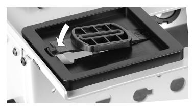
**3-17** Snap the Guides in like this. Use firm pressure just next to the guide latch. Note: The guides are injection molded acetyl and the guide bases may vary slightly in tolerance. **Some may require more pressure to insert.** The tighter guides will become easier after a few insertions.
