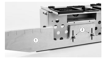
**3-10** The outrigger beam should be <sup>3</sup>/<sub>8</sub>" to <sup>1</sup>/<sub>2</sub>" [10-12mm] plywood, shaped as suggested to minimize weight. Drill and cut out as shown ① and attach using either <sup>1</sup>/<sub>4</sub>-20 [M6] carriage bolts and wing nuts (not supplied) ② or alternatively a pair of optional Leigh F-Clamps ■. See leighjigs.com/support.php#r22
