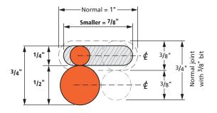
**4-34** The diagram illustrates routing the ¼" joint described above (guide not shown). The result is a perfect ¼" mortise and tenon, ½" smaller both ways than the guide size. Any two bit diameters which add up to two times the nominal guide size will produce a joint the size of the smaller bit. Bear in mind, the maximum usable bit diameter with the Super FMT is ½" [12mm].
