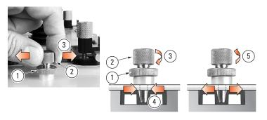
**4-9** Adjust the right hand guide pin. Turn guide pin lock nut ① up under the guide pin ②. Turn the guide pin down ③ until all front-to-back "play" is eliminated ④, then turn it back up ½ of a turn ⑤. To prevent the guide pin from turning, turn guide pin lock nut down firmly against the threaded boss. The router/sub-base should slide freely left to right. Once set, RH guide pin should require no more adjustment.
