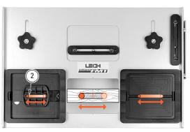
**3-25** Mortises are routed with the guide pin running in the inside mortise slot of the guide ②. Always rout the mortise slightly deeper than the tenon length. Note: In most constructions, only one tenon and perhaps two mortises need to be cross marked and sighted. Please read all of the procedural chapters to gain the utmost efficiency from your Super FMT. ■
