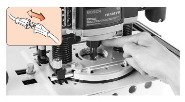
**3-30** Always disconnect the power source from the router when fitting bits, or making adjustments. Before connecting the router to the power source, make sure the bit revolves freely through the sub-base bit hole, and table and clamp plate bit openings in all extreme guide pin positions and preset bit depths.
