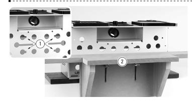
**3-9** The jig clamp plate has four clamp holes with notches ① to allow the mounting of a shop-made mortise beam ② or outrigger beam for handling large mortise pieces for efficient routing of multiple mortises. See Chapter 4, Production Procedures.
