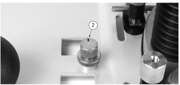
**4-10** Repeat this procedure with the left guide pin set in a guide mortise slot. When you have minimal "free play", use a permanent ink pen to mark a small "dash" at the 12 o'clock position on the guide pin ②. This indexes the guide pin. Before routing your first joint, turn the guide pin up 2 full turns. This is your starting point. Record "number of turns up" or "down" when joint fit is good. Each ½ turn of the LH pin changes the joint glue line fit by approximately 0.0011" [0.03mm].
