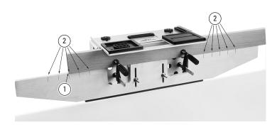
**4-31** Multiple mortises in "ladder" type construction are rapidly routed. Mark all mortises on only one piece (only one of the marks needs a front-to-back mark!). Sight the first mortise (cross) to set the table and mark the top of one outrigger in line with workpiece end ①. Table locked, move workpiece, sighting each successive mortise line, marking the outrigger(s) ②. To rout, align unmarked board ends with outrigger marks ②. ■
