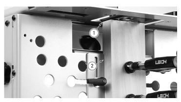
**4-4** Clamp the tenon piece with the end **lightly touching the underside of the sight** ①. Its side edge should touch the previously set sidestop fence ②, with the marked side toward the clamp plate.
