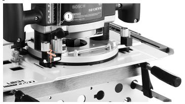
Remove the sight and place the router/sub-base assembly on the jig, the left hand guide pin in the mortise slot part of the guide. Now raise the plunge stop rod ① slightly, say 1/32-1/16"[1-1,5mm] to allow the mortise to be routed slightly deeper than the tenon to ensure perfect tenon shoulder flushness on the finished joint.
