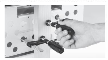
**3-4 Do not over tighten the clamps;** excessive force may damage the workpiece. A few minutes of trial and error testing will soon give you the feel for the correct clamp tension.
