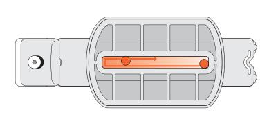
**4-19** Make sure the guide pin is run clockwise against both the front and rear of the mortise guide slot on the final passes. The gap between pin and mortise guide slot is greatly exaggerated in this illustration.
