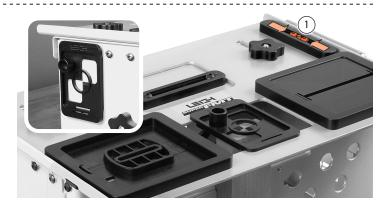
**4-6** Unlock the two **§ FB** front/back limit stops. Move both so they touch the Stop Post, and tighten both stops ①. This prevents front-to-back movement of the table when later sighting the mortise. Remove the sight and store it at the end of the jig.
