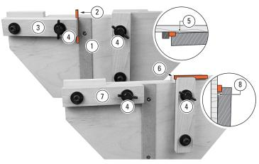
**4-38** To hold very small workpieces ②, make up a rabbeted holder ③ with the rabbet slightly shallower than the workpiece thickness, leaving a gap at ⑤ and ⑧. i.e. For Tenons: Sidestop ① Tenon Piece ② Holder ③ Clamp ④ Gap ⑤. For Mortises: Mortise Piece ⑥, Holder ⑦, Clamp ④, Gap ⑧. ■
