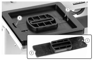
**3-16** Two small projections on the Guide ① fit into undercuts on the right side of the guide recess ②. The left end of the Guide ③ is pushed down and retained by the spring-loaded Guide Latch ④. ⚠ Note: the guide end shapes are not identical. Guides can only be installed one way as shown here.
