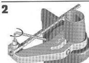
Install clamp bracket on end of rod. Some routers, (e.g. Bosch 1613) may require use of supplied rod adaptor. See 3.
