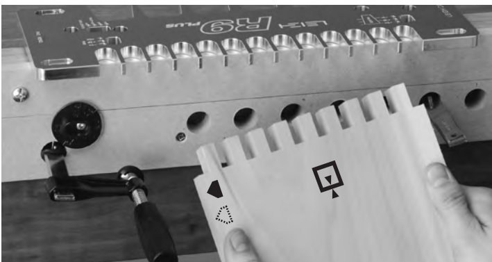
2-2 Box joint boards are clamped against the beam both "face in" and "face out" for alternate end cuts. With box joints, the same side edge always goes against the sidestop.
