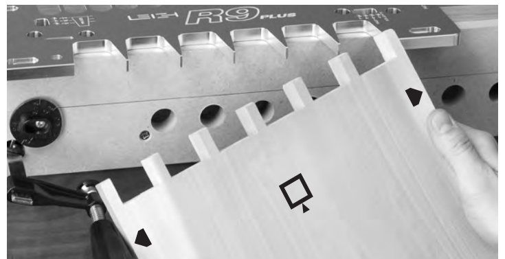
2-3 Note: Because through dovetail pin and tail boards face only one way, both side edges are (alternately) used against the sidestop. ■
