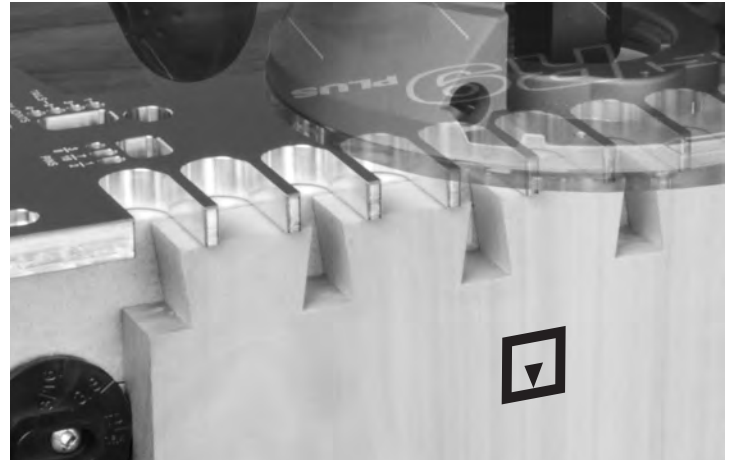
2-1 Icons such as the one above indicate which side of the board faces out (toward you, the operator) when clamped in jig, and which faces are in or out when assembled.
