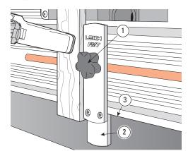
The FMT's newly designed side stop fence is attached in all modes by a single knob and T-bolt inserted to the centre clamp plate slot ①. Most tenon pieces are routed vertically, and for that purpose the short part of the fence 2 acts as a T-square against the edge of the clamp plate 3. In this mode the Leigh logo faces toward you.
