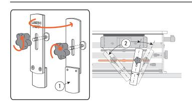
Angled Joints: Remove the knob and T-bolt. Reverse the fence so the short end faces toward you ①. The fence may now be set at any angle along the centre clamp plate slot ② by tightening the knob.
