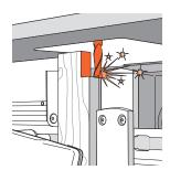
WARNING: Never rout tenons with the side stop fence in the inverted position (with the short end up in the cutter opening). The inverted fence mode is only used to support small mortise stock.
