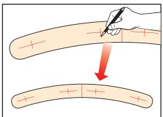
On flat curved surfaces such as this where the mortise is not automatically parallel to the clamp plate, make sure you extend the long axis mortise centreline mark to extend well beyond the mortise area.
