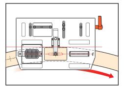
Rout mortise, release clamps and move workpiece to sight the next mortise axis guide lines. Adjust the table as necessary for each mortise.
