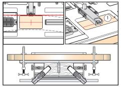
Mount your shop made auxiliary bracket to the FMT and "sandwich" the mortise board under the table. Adjust the workpiece so that the long joint axis line is parallel to the jig; either by measurement or by aligning with the two centreline marks in the table opening ① (later model FMTs)
