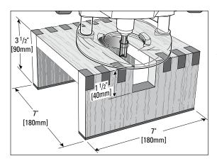
**12-4** Router Stand: Make up a small router stand as illustrated, to mount the router securely on the bench when not in use.
