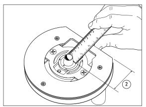
**7-4** Measure the distance from the guidebush to the rear edge of the router base ②.
