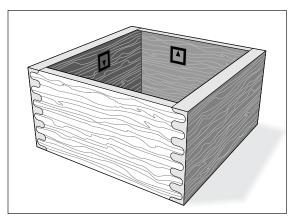
**7-16** Assemble in the usual way. You will probably need to clamp in both directions when gluing up.
