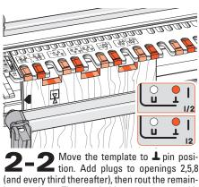
(and every third thereafter), then rout the remaining openings. The very bold among you can skip adding the extra plugs and after moving to the  $\bot$  position, rout only the template openings to the left of each plug
