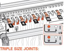
**2-1** Board 1: Plug openings 1, 4, 7, 10 and 13 (i.e. every third opening thereafter). Set the template in the **U** pin position and rout all of the open sockets in board 1. Do not move the board.
