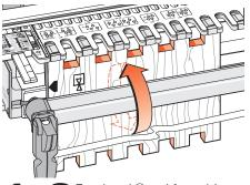
**1 – 8** Turn board <sup>①</sup> end-for-end (same side edge to the side stop and opposite face against the jig each time). Repeat steps 6 and 7 on this end of board <sup>①</sup> and on both ends of board <sup>③</sup>.
