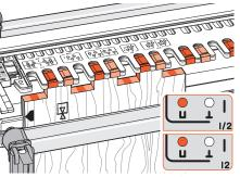
**2-4** Move the template to **U** pin posiings numbers 2, 5, 8 (and every third opening thereafter). Again, those with their wits about them can skip adding the extra plugs and after moving to the **U** position, rout only the template opening to the **right** of each plug.
