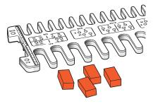
**1**-**1** These procedures require you to rout into some template comb openings and not others. You will need to make "plugs" to block some openings in the selected comb. These are very simple and quick to make on your table or band saw.
