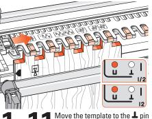
**1 – 1 1** position and again, rout all of the open sockets in board 2
