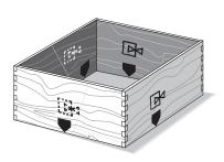
**1–13** Assemble the box with all of the four "side-stop edges" either at the top, or at the bottom of the box.
