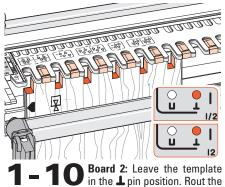
odd numbered template openings in board 2. Do not move the board.
