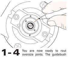
adjustment for joint fit on oversize joints should be exactly as it was for the nominal size, **but rout a test oversize joint first to confirm the fit**.
