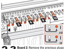
**2-3** and plug openings **3**, **6**, **9**, **12** and **15** (i.e. every third opening thereafter). With the template still in the **1** pin position, rout all of the open sockets in board 2. **Do not move the board.**
