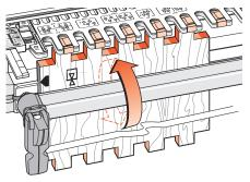
**1-12** Turn board 2 end-for-end (don't forget, the same side edge to the side stop) and repeat steps **10** and **11** on this end of board **2** and on **both ends of board 4**.
