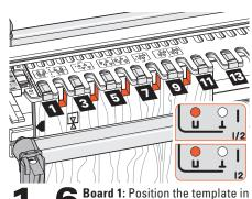
**1 – 6** Board 1: FOSITION and Compared the Upin position. Rout in the even numbered template openings across one end of board (1). Do not move the board.
