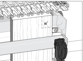
13 Remove the boards from the left side of the jig. Make sure the support brackets are still in the fully raised position. Temporarily re-install the finger assembly onto the support brackets (any mode). Repeat the sidestop bumper setting procedure with the lath, on the front right side of the jig. Then remove the finger assembly and repeat the alignment procedure for the rear right sidestop with the second board.
