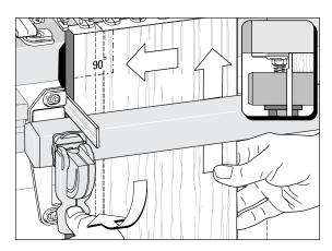
**8** With the lath trapped in place, clamp the board.
