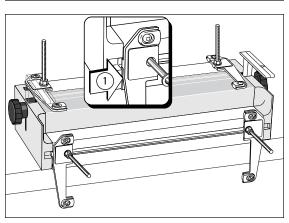
**3** Position the side stops with the outer edge of the **casting** flush with the ends of the extrusion ①. Firmly tighten the nuts until the side stops are seated.
