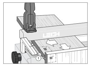
**10** Remove the finger assembly. Place the second 90° test board under the rear clamp, front end edge flush against the front board. Slide the rear board side to side until the left side edges are flush ①.
