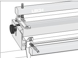
**5** Place four springs and two clamp bars on the T-bolts. The large holes in the clamp bars go right over the springs. Make sure the clamp bars move freely on the T-bolts. The Leigh logo or decal should be on the rear (upper) clamp bar facing you.
