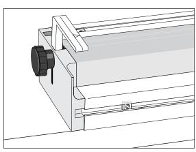
1 Remove the finger assembly, cam clamps or clamp knobs, clamp bars, side stops and bolt assemblies. Reassemble the T-bolts, nuts and washers with the new stops as shown.
