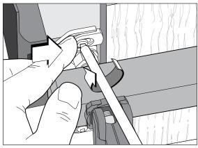
**9** Remove the lath and loosen the bumper setscrews. Slide the top bumper against the board and tighten the screw firmly. Position and tighten the bottom bumper.
