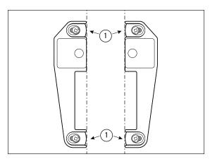
4 Note that the adjustable bumpers ① are factory set in the retracted position, which is set back from the main body of the sidestop. This is for setup alignment purposes. If yours are not in this position, make sure that they are before proceeding. Remount the finger assembly with support brackets in fully raised position.
