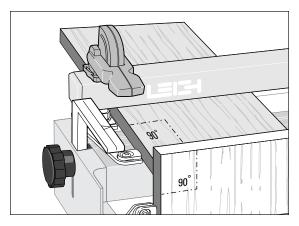
**12** Clamp the rear board (if you have cam clamps, by pulling the lever forward this one time only so that the rear bumper screw is accessible). Position the bumpers against the top board and tighten the setscrews.
