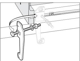
**2** Insert two T-bolt/sidestop sub-assemblies into each of the two main extrusions. Make sure the side stop, washer, and nut are in the correct order as illustrated, with the locating lugs engaging in the extrusion slot. Note: The lugs will be tight to enter the extrusion slot, but the nut will force the lugs in. See step 3 before tightening.
