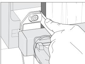
7 To set the sidestop bumpers, adjust the clamps to receive the two square boards. Use the end of the lath to position one of the 90° test boards away from the front left hand sidestop casting. Make sure the top end edge of the board is touching flush under the guide fingers.
