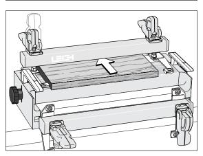
14 D1258 jig owners: Make up a spacer board to support the finger assembly in all front-clamping vertical board modes. The spacer board should be flat, straight and of even thickness. We suggest <sup>3</sup>/<sub>4</sub>" x 6" by approximately 11½" or 23" long, depending on your jig size. This is to keep the finger asembly above the rear side stops. D1258R and D3 jig owners should already have their spacer boards made.
