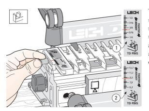
Where finger assembly scales overlay an illustration, the "inches" scale ① will be at the top, the "millimetres" scale ② will be at the bottom. Only the front "active" half of the scales are illustrated. For clarity, setting positions are indicated with a red line in the manual only. On the jig, the lines are black.
